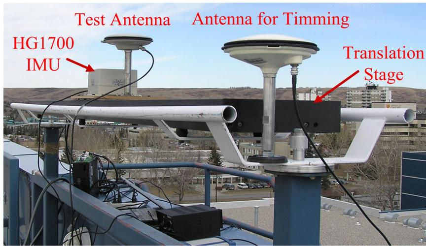
**Figure 4.5 Translation Stage Test Setup**
