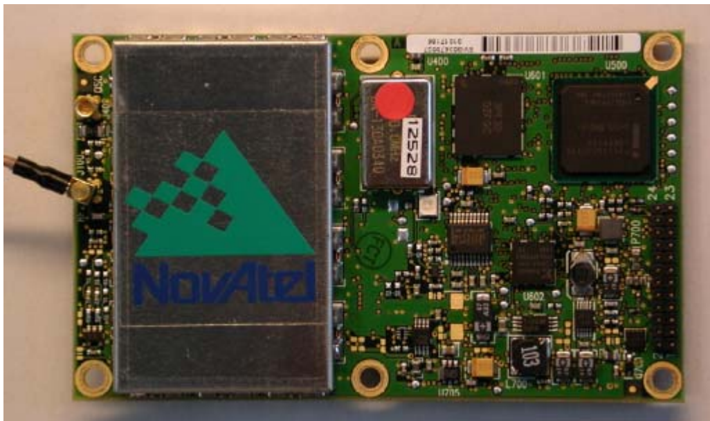
Figure 4-1: NovAtel OEM4-G2L Dual-Frequency GPS Receiver (125X85 mm) (OEM4-G2L, 2003)
