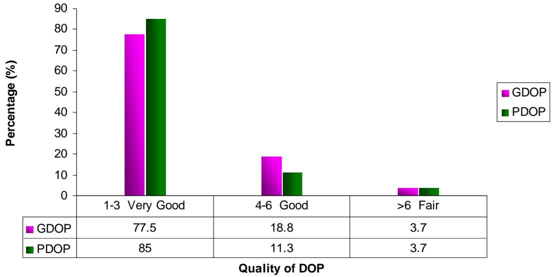
**Figure 5-22: Analysis of DOP for Zero deg Elevation**
