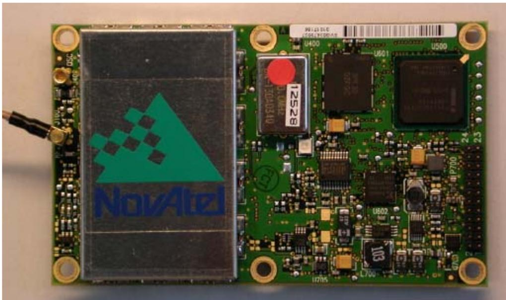
**Figure 4-1: NovAtel OEM4-G2L Dual-Frequency GPS Receiver (125X85 mm)
