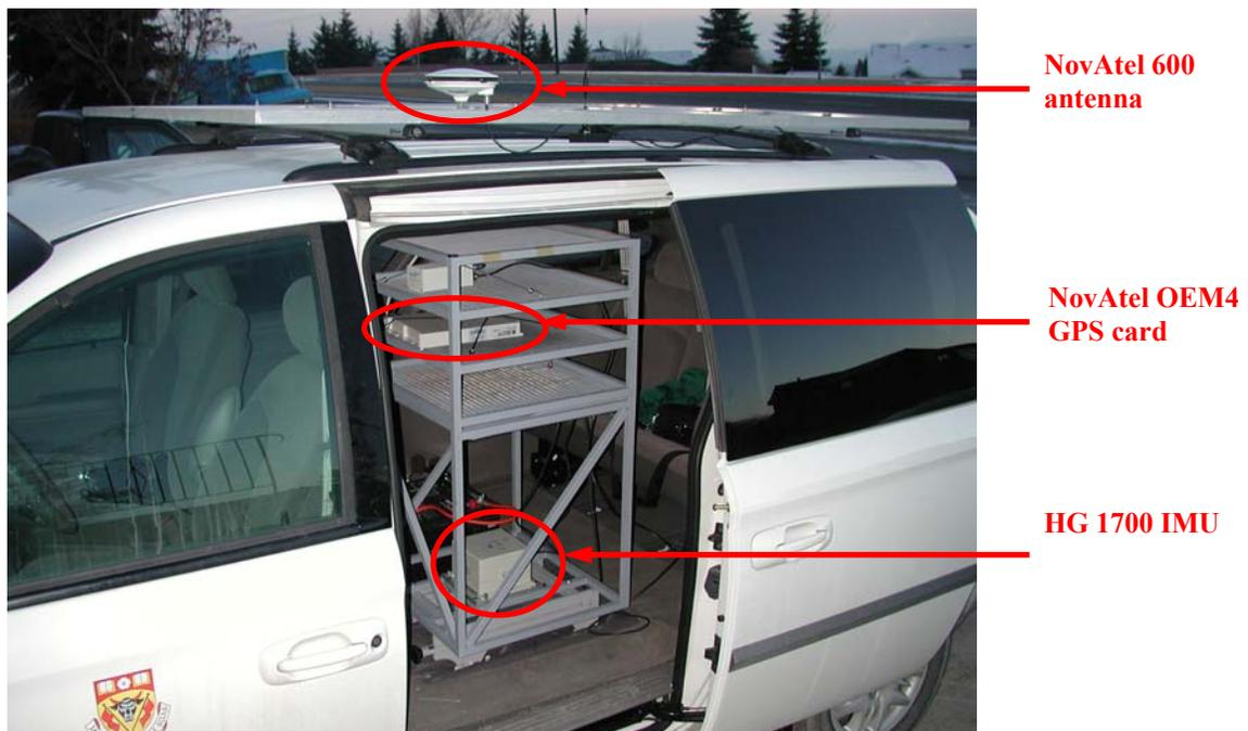
**Figure 6-2: Remote Station Set-up**
