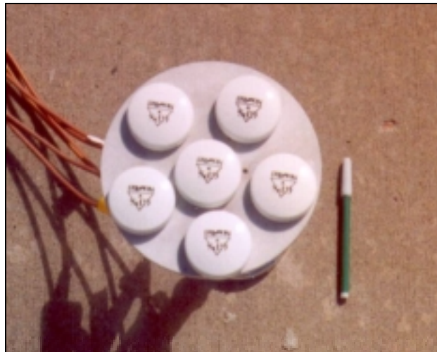
Figure 7.1: Multi-antenna array assembly
