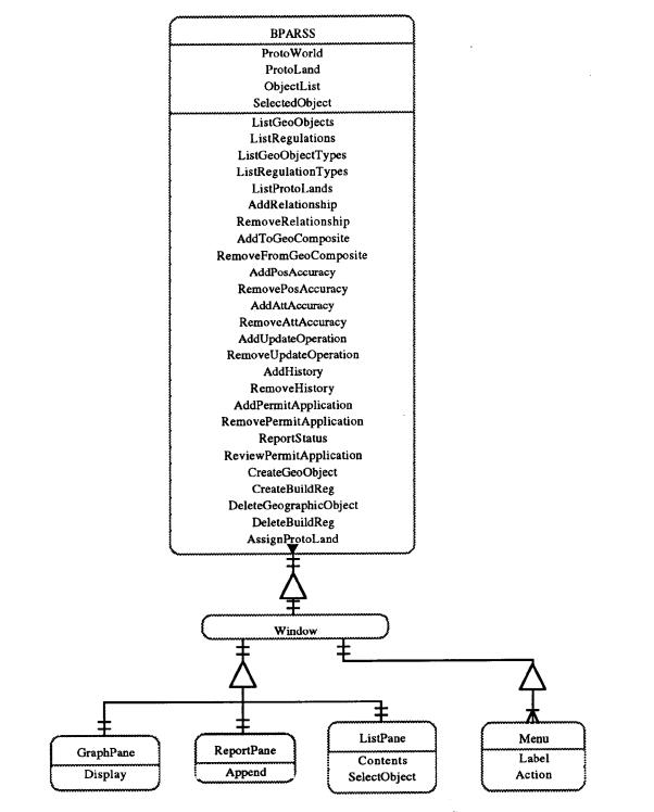
Figure 5.2.2 Human Interaction Component Structure
