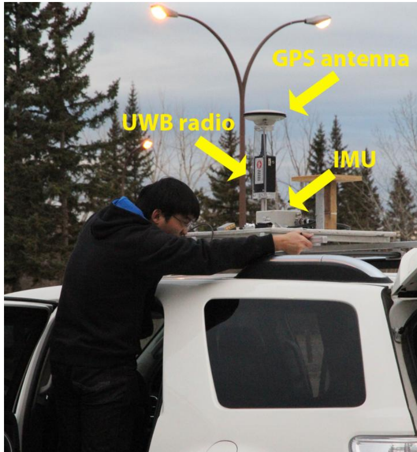
Figure 4.2 GPS antenna, UWB, and IMU equipment setup on the test vehicle
