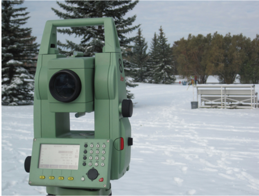
Figure 5.1: Leica TCR803 total station, used during the in the initial creation of the survey network and establishment of the truth coordinates.
