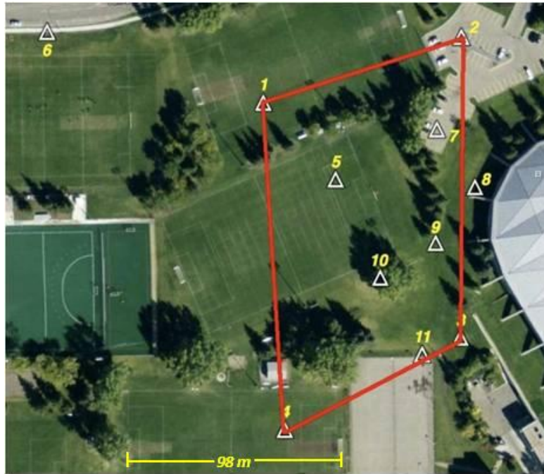
Figure 5.4: The various points (marked by triangles) that make up the survey network, and the localization area (marked in red).
