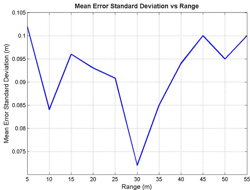
**Figure 5.11:** Mean error standard deviation values for indoor testing of MSS radio
