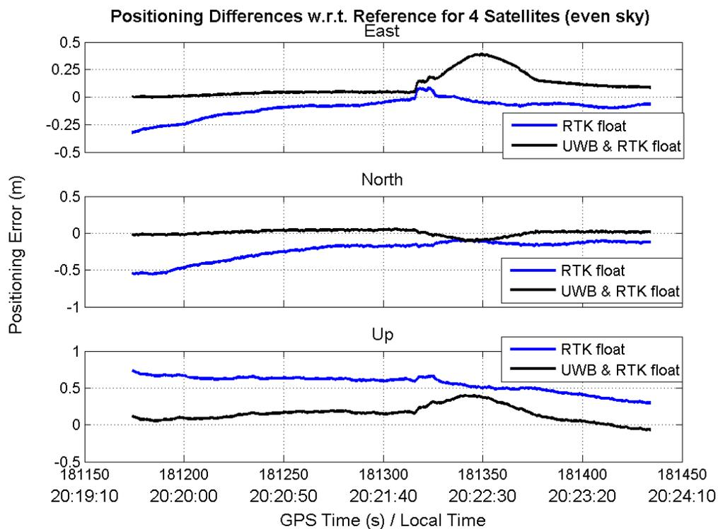
**Figure 7.25:** Positioning differences between the reference solution and RTK float with and without UWB augmentation for the “good” signal case
