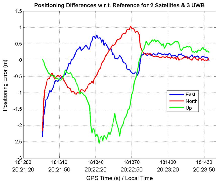
**Figure 7.33:** Positioning differences between reference and the 2 Satellites & 3 UWB solution.
