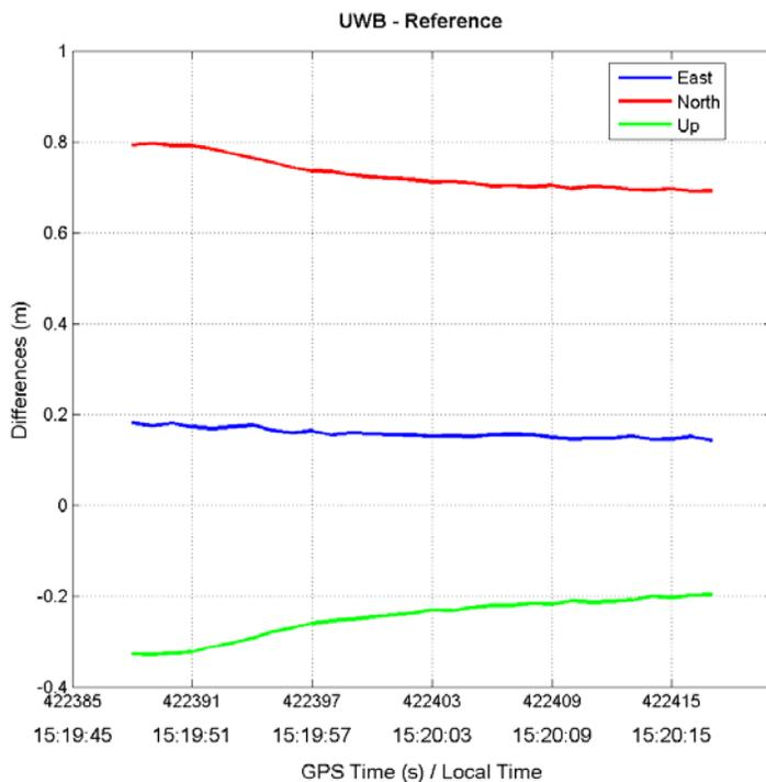
**Figure 6.6:** Difference between the UWB solution and GPS RTK float solution for rover site #1
