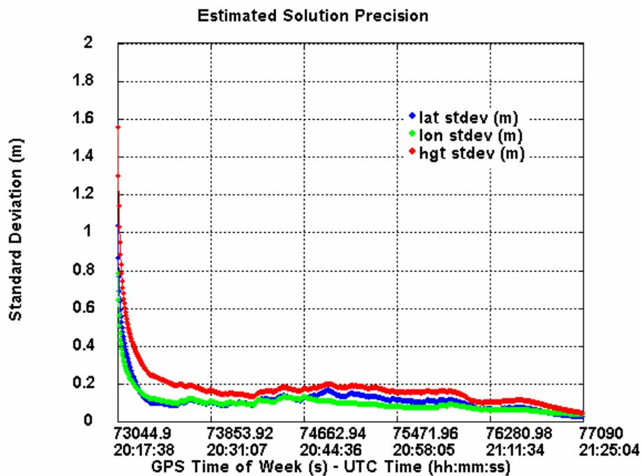
Figure 7.10: Standard deviation for the GPS-only solution
