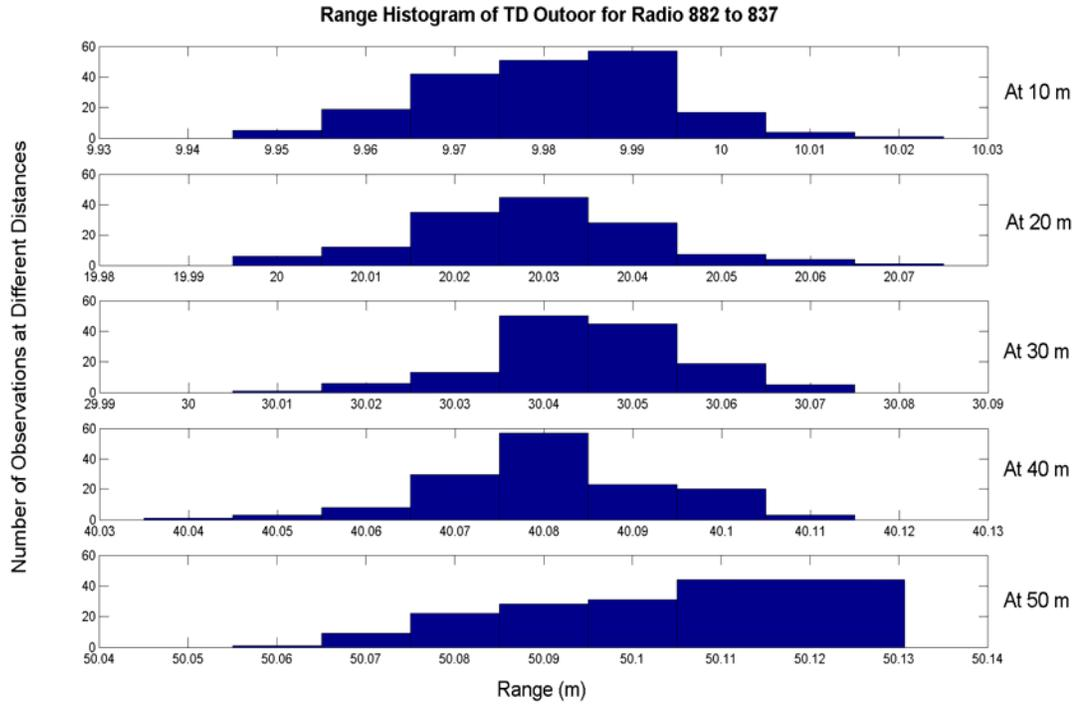
**Figure 5.16:** Range histogram between TD radios 882 to 837, outdoors
