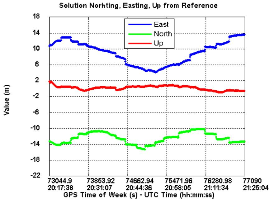
Figure 7.8: Float position solution for GPS-alone
