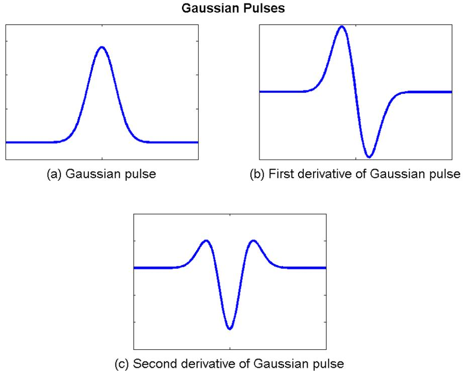
**Figure 3.1:** (a) Gaussian pulse in time domain; (b) the first derivative of the Gaussian pulse, also known as the Gaussian pulselet; and (c) the second derivative of the Gaussian pulse
