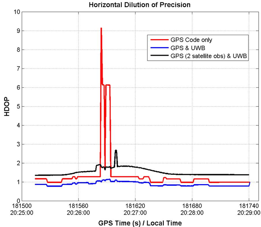
**Figure 6.29:** HDOP for various positioning schemes [kinematic]
