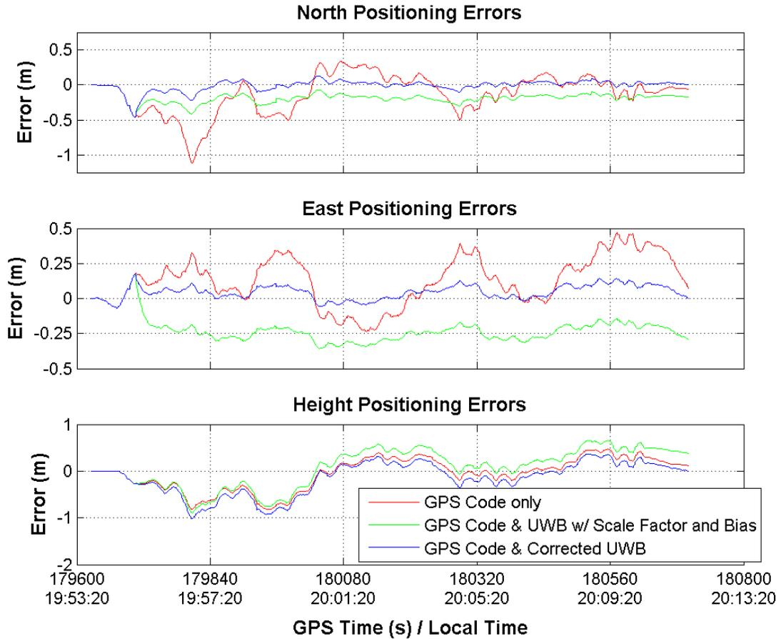
**Figure 6.25:** Positioning errors for various processing schemes [static]
