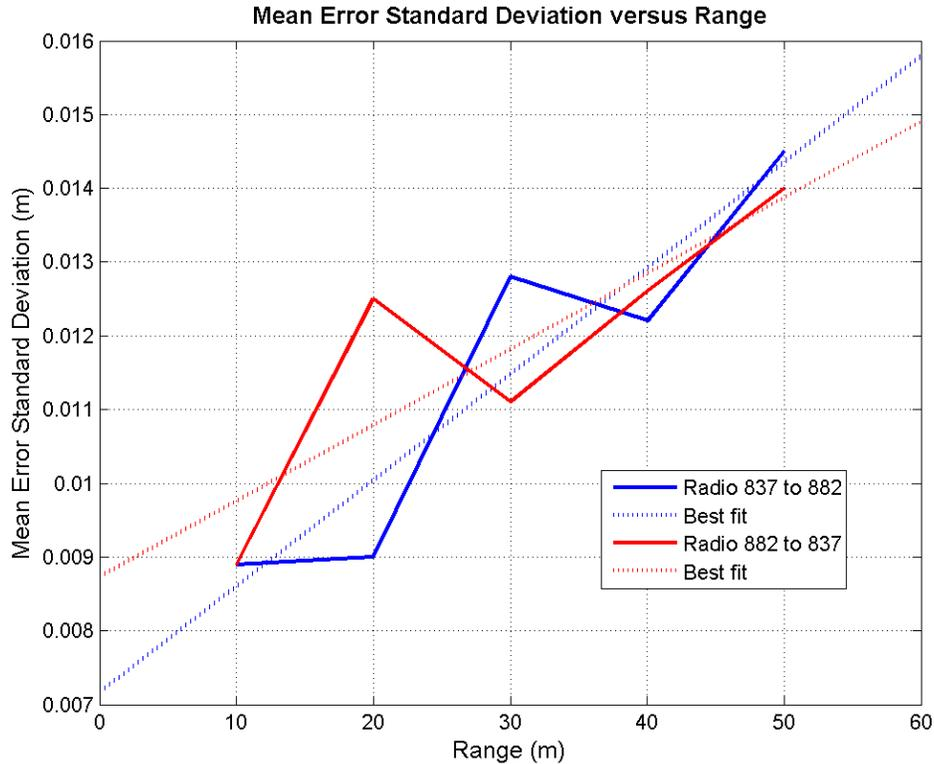
**Figure 5.19:** Mean error standard deviation for two TD UWB radio combination pairs, outdoors
