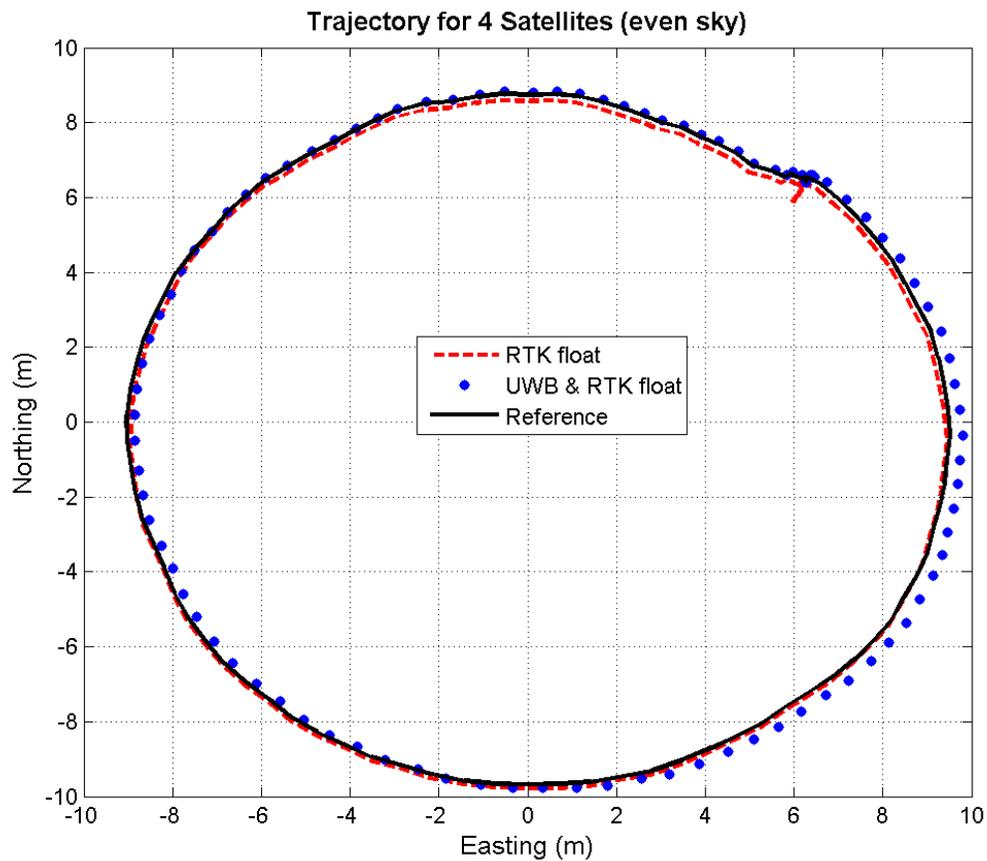
**Figure 7.26:** Trajectory for the “good” scenario
