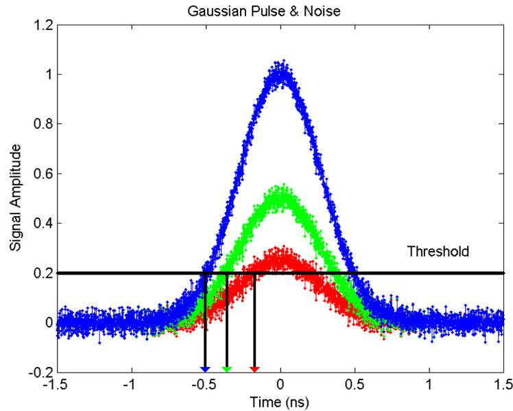
**Figure 5.32:** A geometric delay error is induced as signal power and amplitude decrease and as result, pass the threshold value at a delayed time
