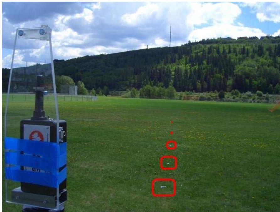
**Figure 5.13:** A soccer field at Shouldice Park in Calgary, Canada. Outdoor testing of TD and MSS UWB radios is done on the soccer field.
