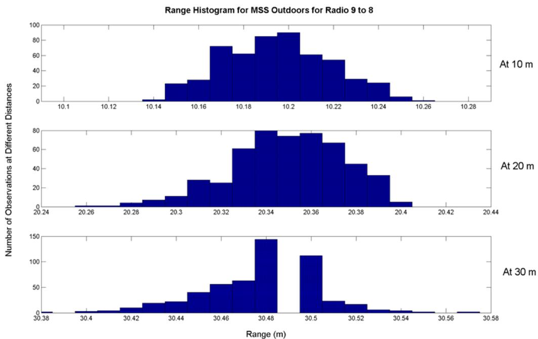
**Figure 5.25:** Range histogram of MSS radii 9 to 8 at different ranges, outdoors
