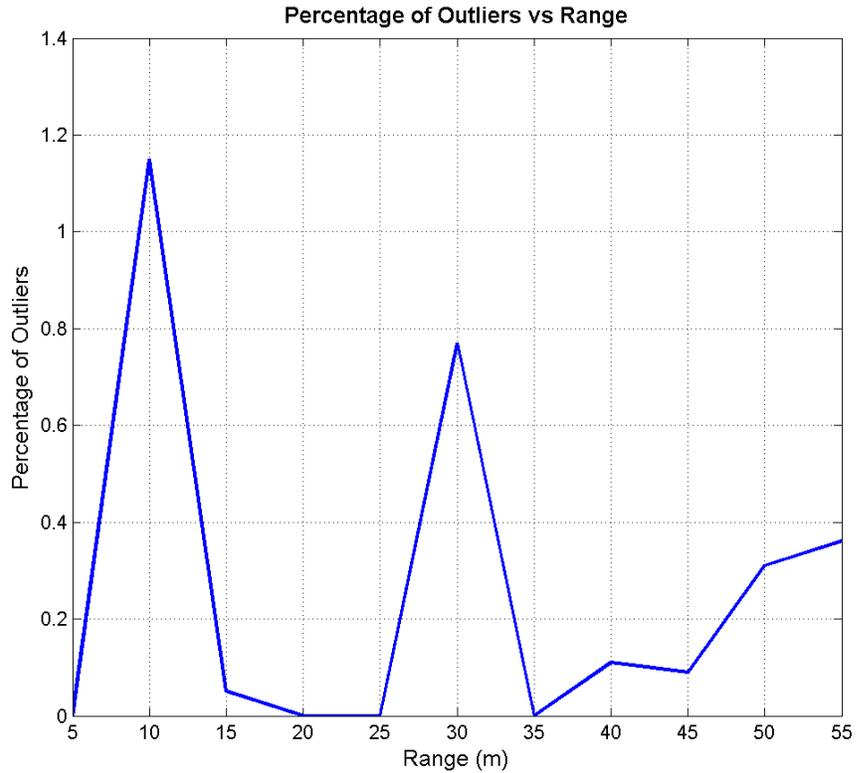
**Figure 5.9:** Number of outliers versus distance for indoor MSS radios
