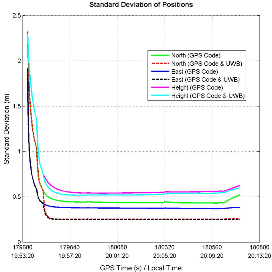
**Figure 6.26:** Standard deviation for position solutions [static]
