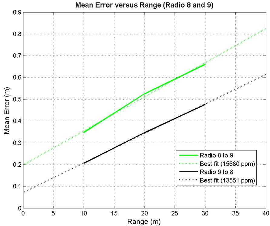
**Figure 5.29:** Mean error values for MSS radios 8 and 9 tested outdoors
