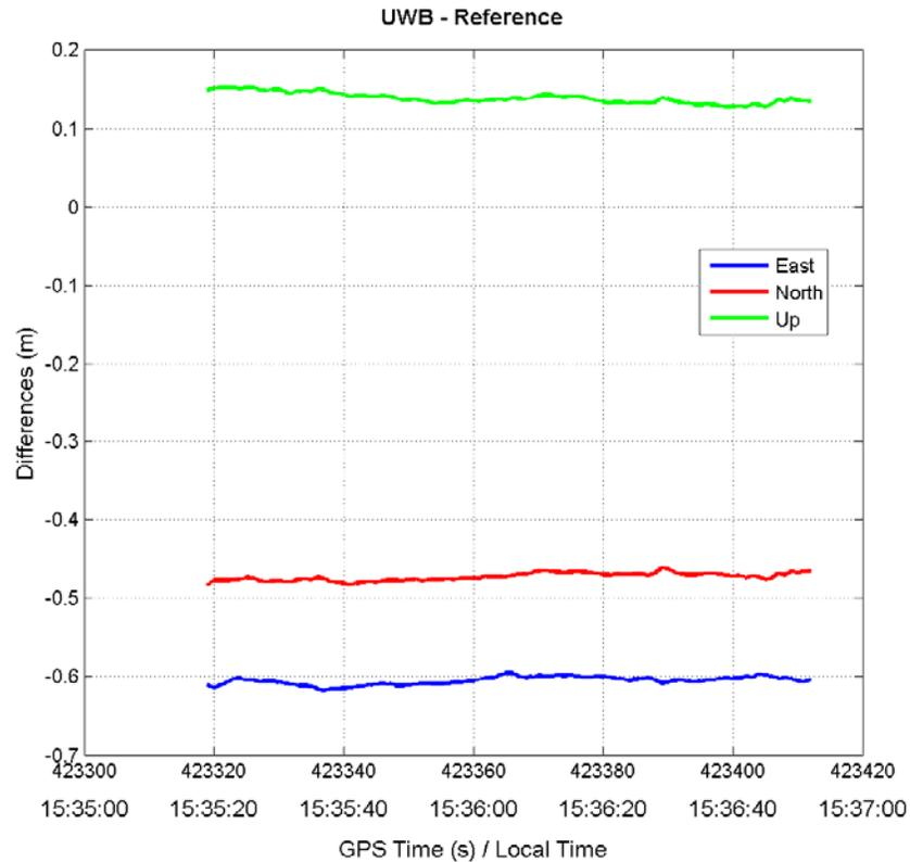
**Figure 6.9:** Difference between the UWB-only solution and GPS RTK float solution for rover site #2
