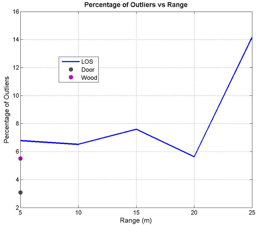
**Figure 5.3:** Percentage of outliers removed from the data for TD measurements.
