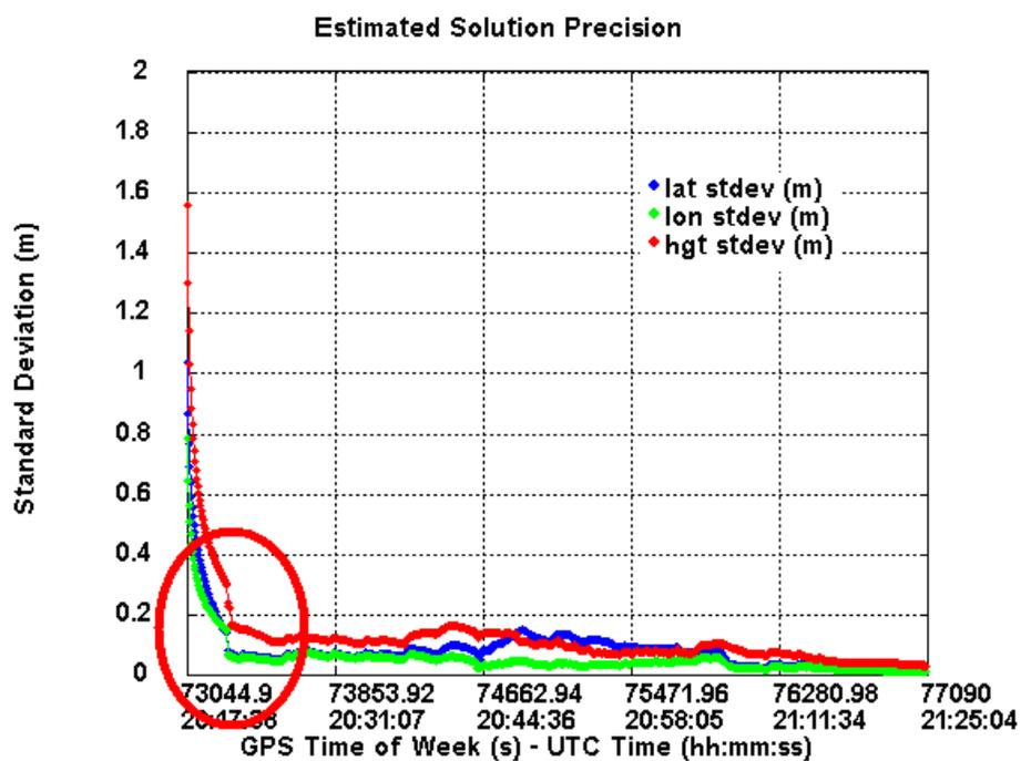
Figure 7.11: Standard deviation for the UWB-GPS solution. Red circle represents the time when UWB is introduced into the Kalman filter.
