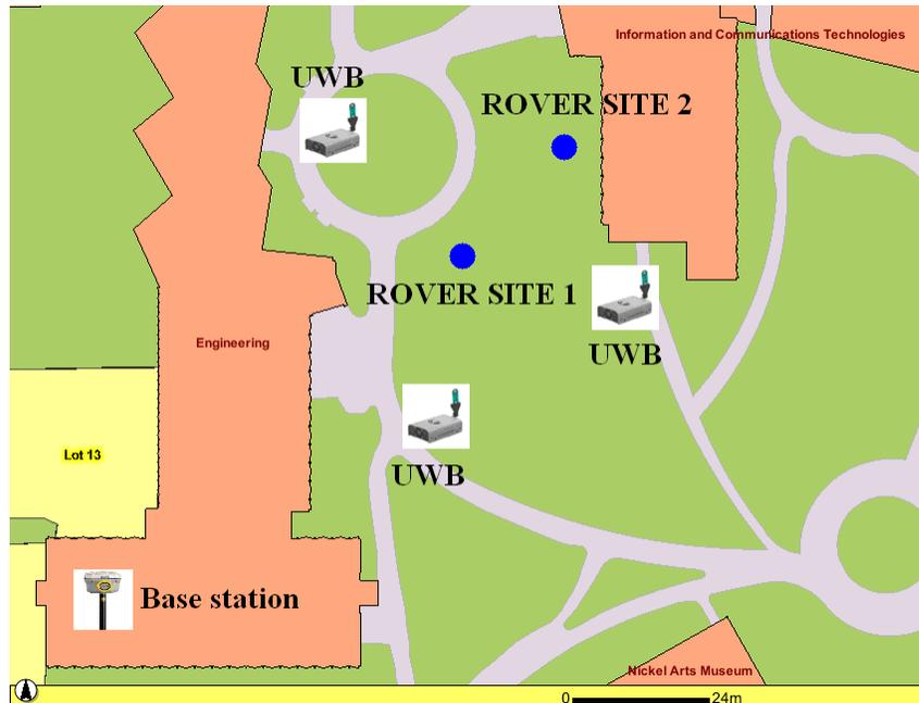
**Figure 6.4:** Digitized view of test area. One base station, three UWB radio tripods and two different rover locations for testing are shown (from University of Calgary 2008)
