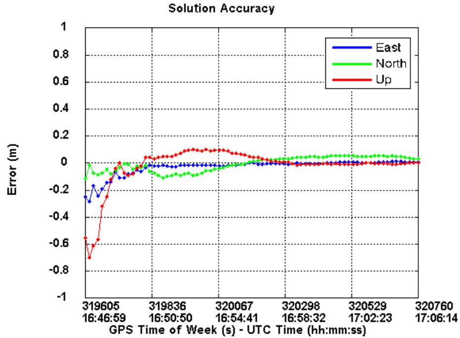
**Figure 7.1:** Position Errors for GPS-alone solution
