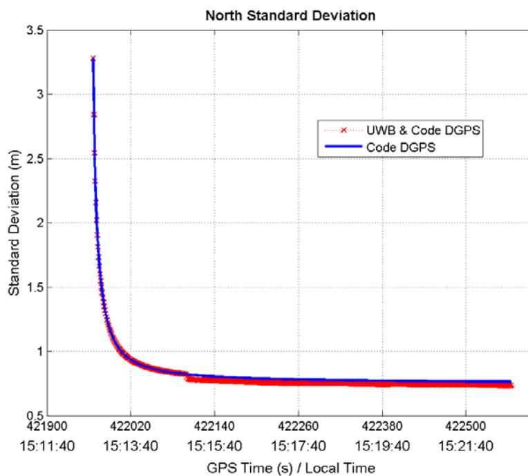
**Figure 6.13:** North standard position for single range UWB augmented to code DGPS, compared to code DGPS alone, for rover site #1
