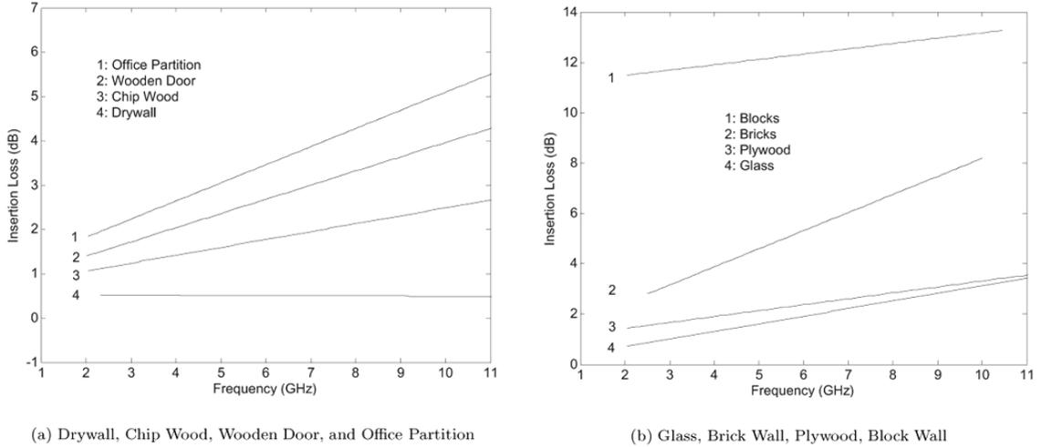
**Figure 3.5:** Attenuation loss for UWB through typical indoor building materials (from Reed 2005)
