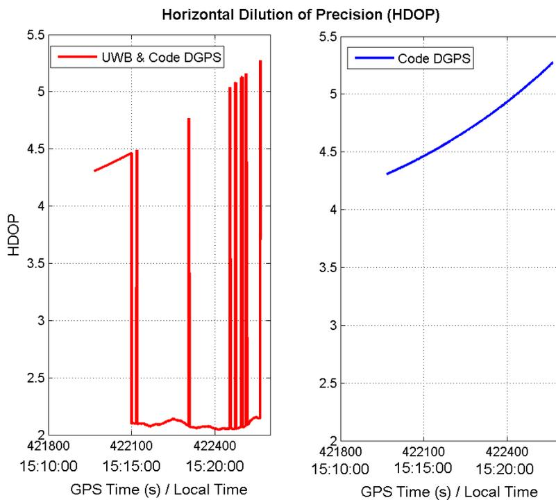
**Figure 6.15:** Horizontal DOP for single range UWB augmented to code DGPS, compared to code DGPS alone, for rover site #1
