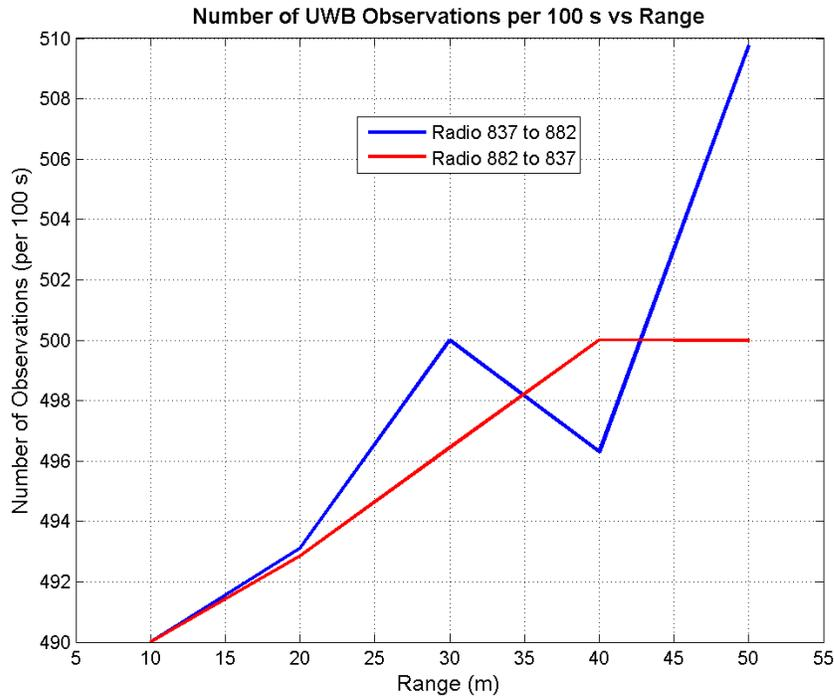
**Figure 5.14:** Number of observations made per 100 seconds for two combinations of TD UWB radios, outdoors
