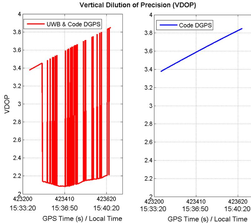
**Figure 6.21:** Vertical DOP for single range UWB augmented to code DGPS, compared to code DGPS alone, for rover site #2
