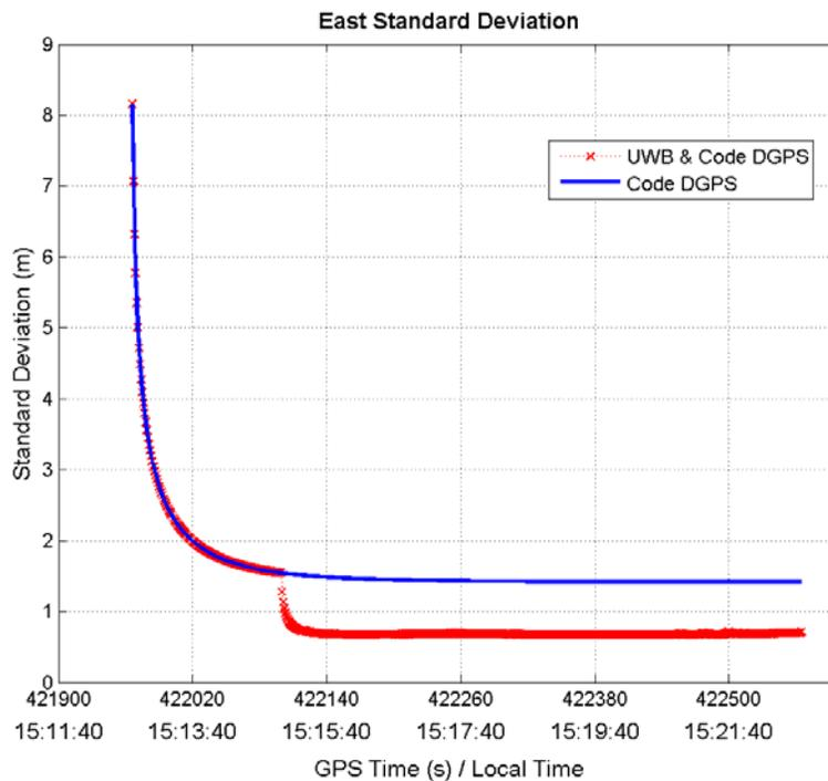
**Figure 6.12:** East standard position for single range UWB augmented to code DGPS, compared to code DGPS alone, for rover site #1
