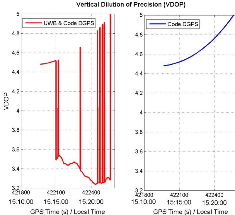
**Figure 6.16:** Vertical DOP for single range UWB augmented to code DGPS, compared to code DGPS alone, for rover site #1
