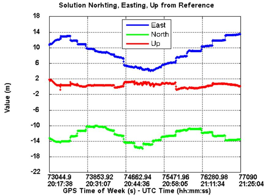
**Figure 7.9:** Float position solution with UWB augmentation
