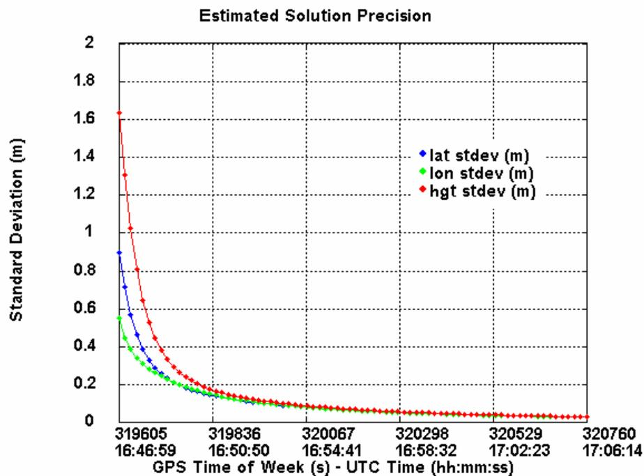
Figure 7.3: Standard deviation for GPS-alone solution
