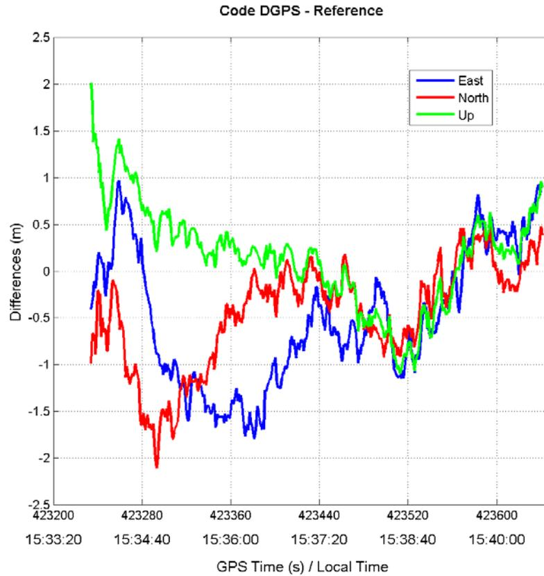
**Figure 6.10:** Difference between the code DGPS solution and GPS RTK float solution for rover site #2
