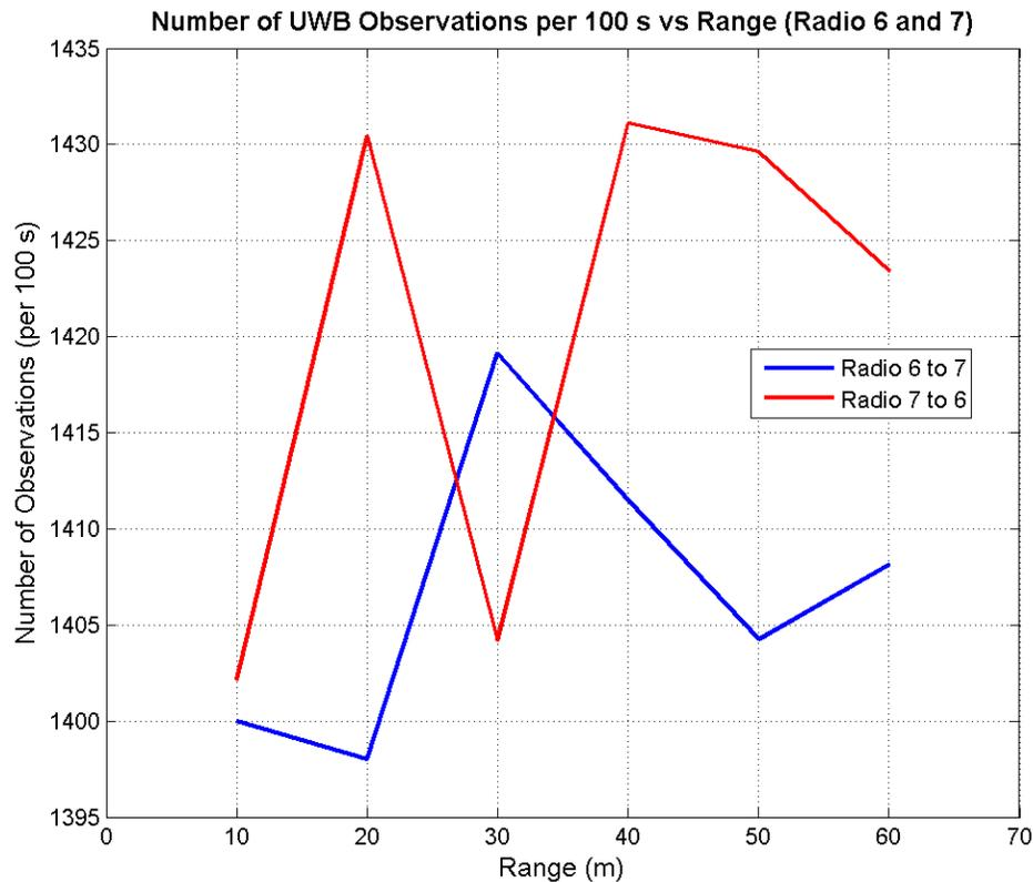
**Figure 5.20:** Number of observations made for MSS radios 6 and 7 per every 100 s, outdoors
