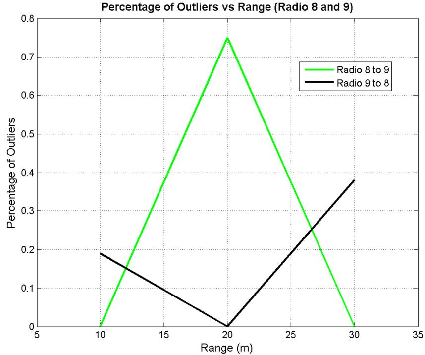
**Figure 5.27:** The percentage of outliers removed from MSS radios 8 and 9
