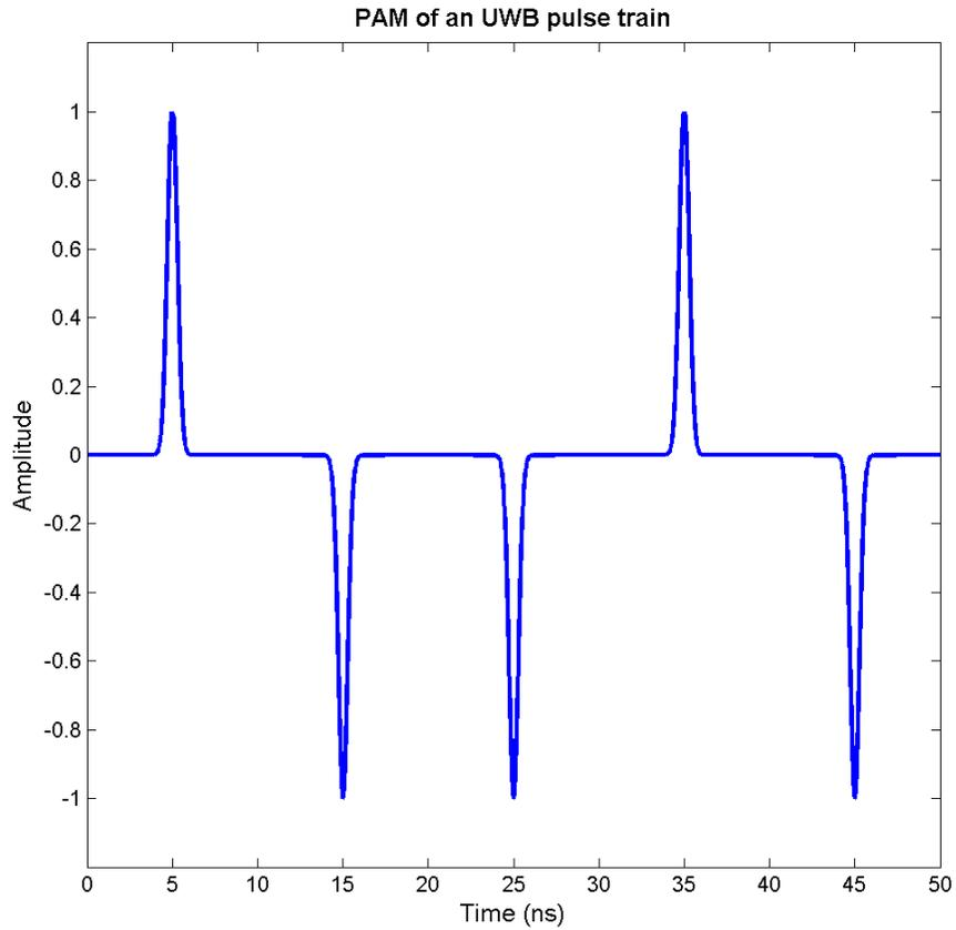
**Figure 3.3:** Pulse Amplitude Modulation of an UWB pulse train
