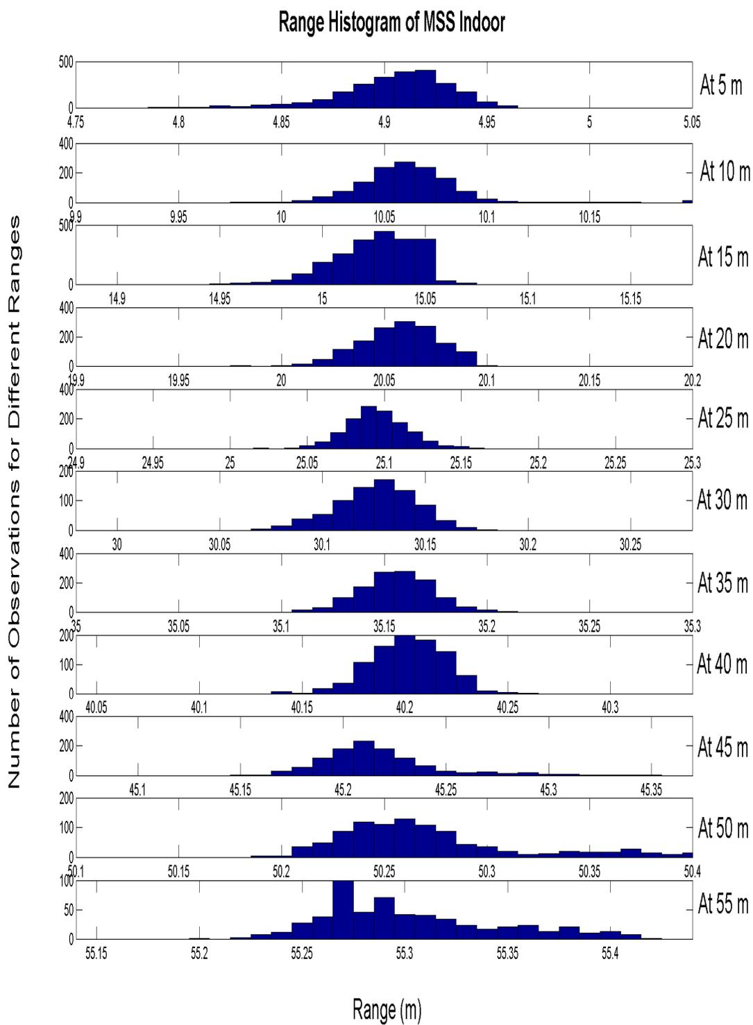
**Figure 5.8:** Range histogram for MSS radios, indoors
