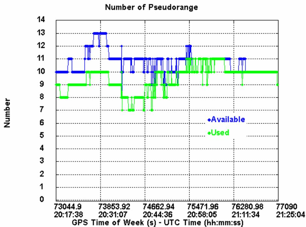
Figure 7.7: Number of satellites available (pseudorange and phase measurements are used)
