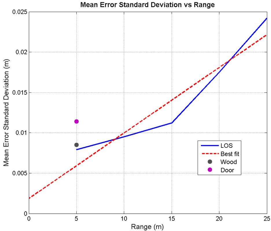
**Figure 5.5:** Mean error standard deviation values for TD indoor measurements. Measurements through the door and wood are NLOS.
