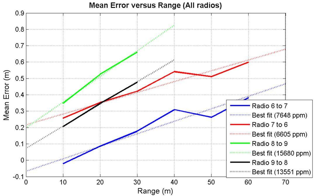
**Figure 5.30:** Mean error values for MSS radios tested outdoors
