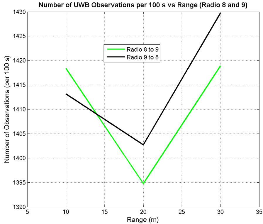
**Figure 5.21:** Number of observations made for MSS radios 8 and 9 per every 100 s, outdoors
