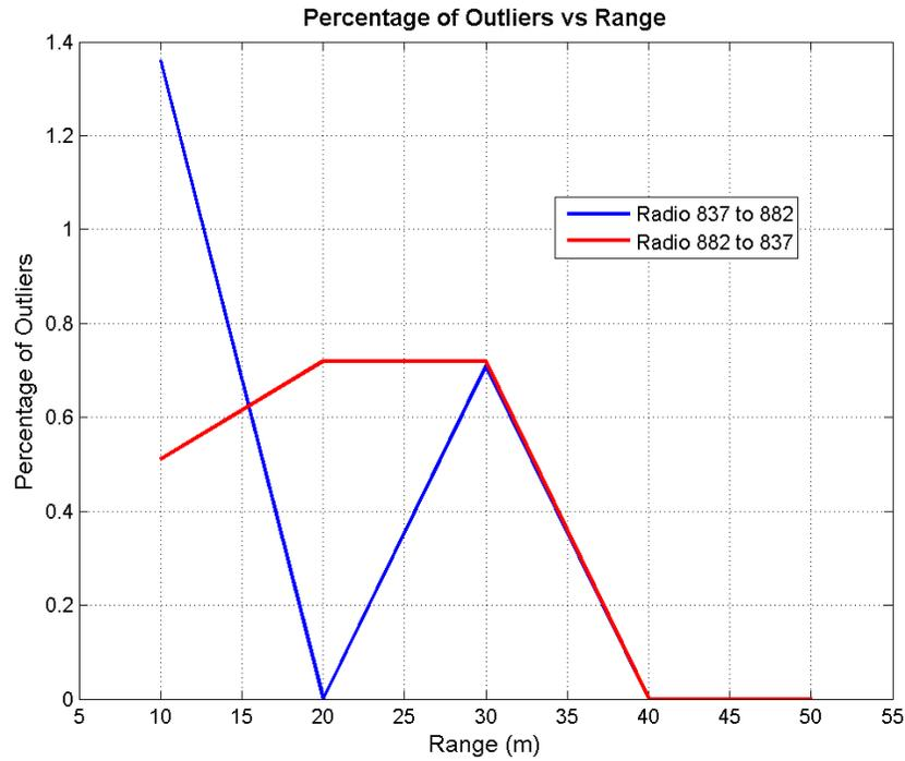
**Figure 5.17:** Percentage of outliers removed from data for two combinations of TD UWB radios, outdoors
