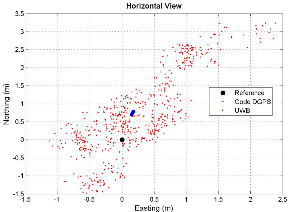
**Figure 6.8:** Plane view for the UWB, code DGPS, and GPS RTK float position solutions for rover site #1
