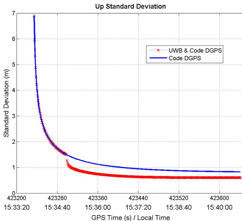
**Figure 6.19:** Up standard position for single range UWB augmented to code DGPS, compared to code DGPS alone, for rover site #2
