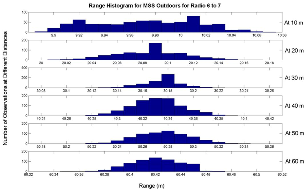
**Figure 5.22:** Range histogram of MSS radios 6 to 7 at different ranges, outdoors
