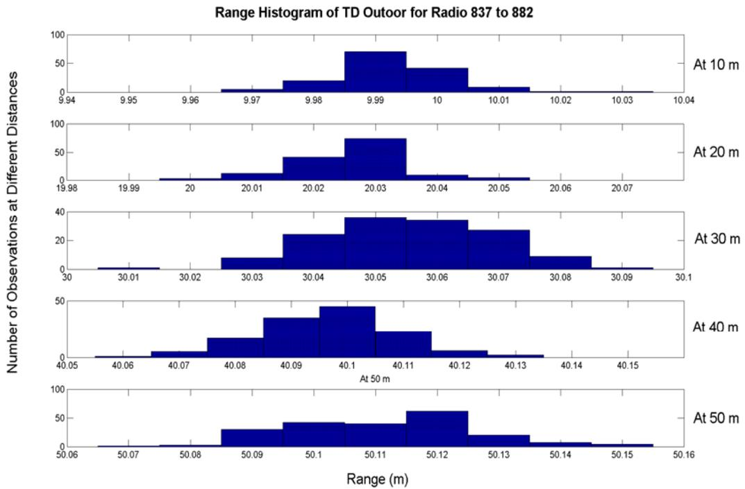
**Figure 5.15:** Range histogram between TD radios 837 to 882, outdoors
