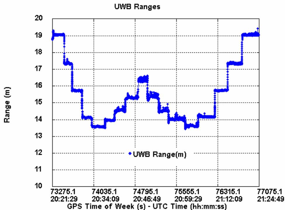
Figure 7.6: Observed UWB range as a function of time
