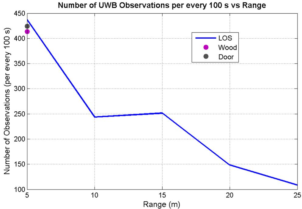
**Figure 5.1:** Number of measurements made by the TD radio per every 100 seconds plotted against range. The blue line indicates LOS measurements, while the purple and black dot represent measurements made through a piece of wood and door, respectively.
