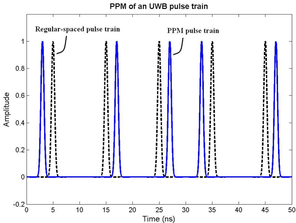
**Figure 3.4:** Pulse Position Modulation (PPM) of a UWB pulse train. The black dashed line is a regularly spaced pulse train, while the blue solid line represents the PPM of the same pulse train.
