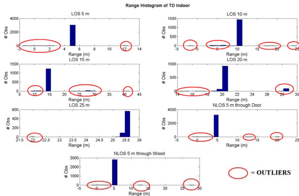
**Figure 5.2:** Range Histogram of Time Domain UWB radios indoors. The red circles are outliers.
