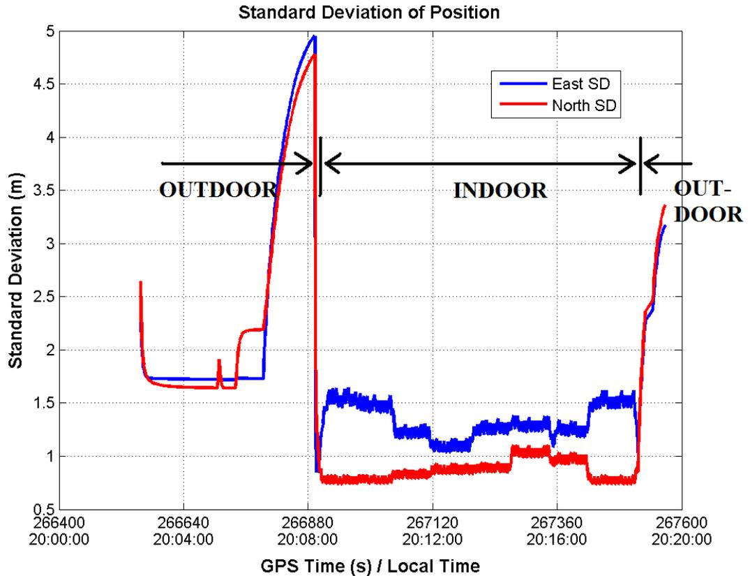
**Figure 6.35:** Standard deviation of positions for outdoor-indoor test
