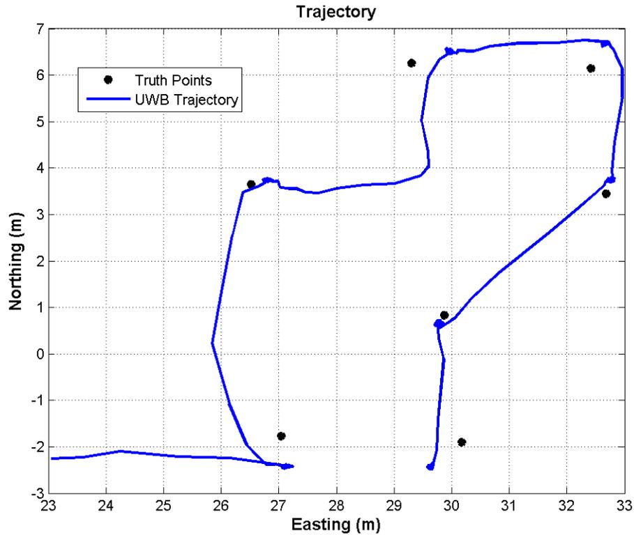
**Figure 6.34:** Indoor UWB trajectory versus truth points
