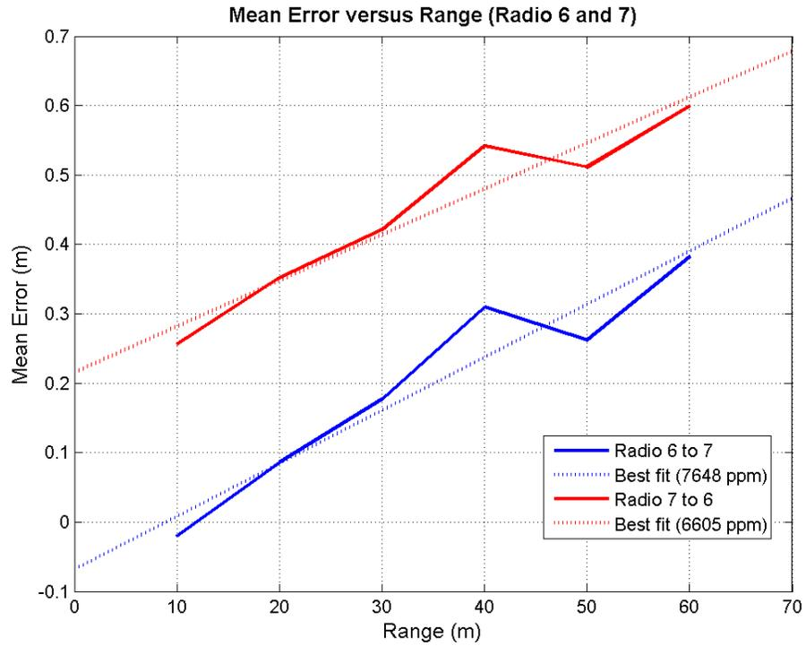
**Figure 5.28:** Mean error values for MSS radios 6 and 7 tested outdoors
