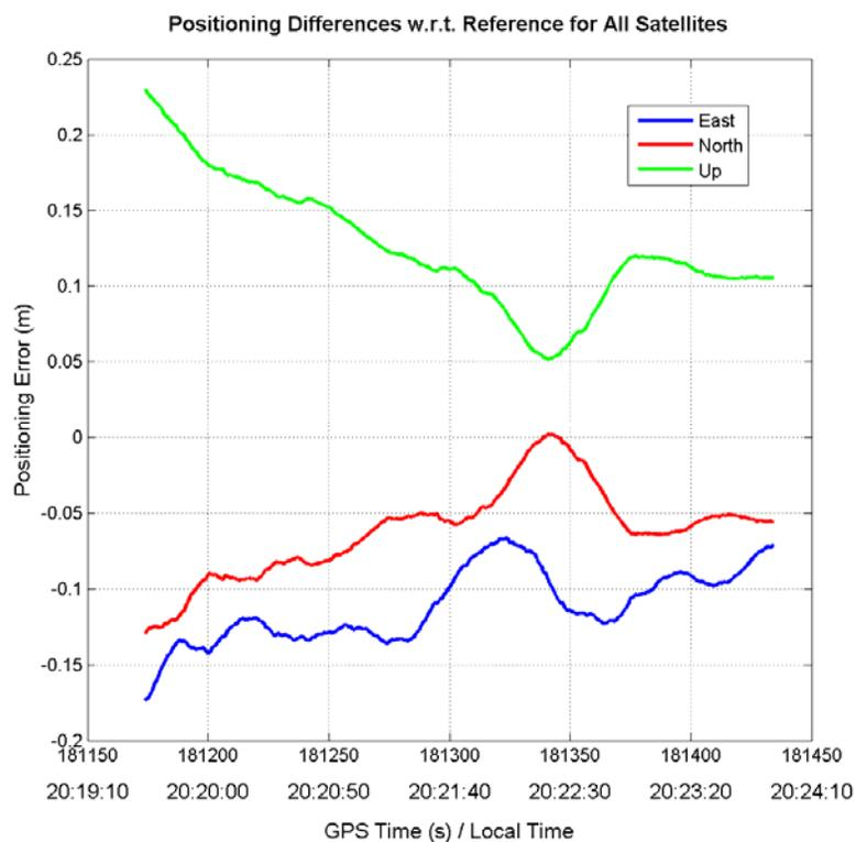
**Figure 7.21:** Positioning differences between all satellites solution with reference. The reference solution is chosen to be the all satellites solution augmented with 3 UWB ranges.
