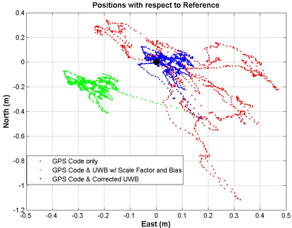
**Figure 6.24:** Position solutions for various processing schemes. The black dot is the reference truth point. [static]
