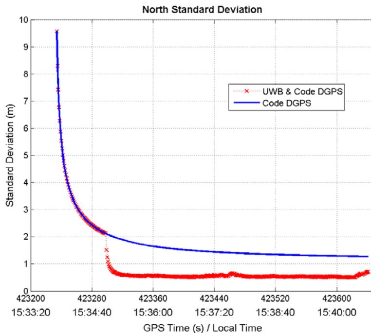
**Figure 6.18:** North standard position for single range UWB augmented to code DGPS, compared to code DGPS alone, for rover site #2
