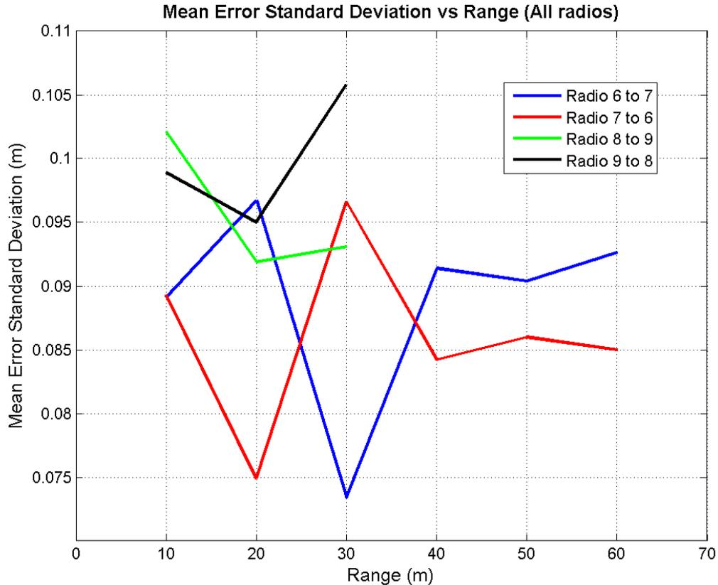
**Figure 5.31:** Mean error standard deviation for MSS radios outdoors
