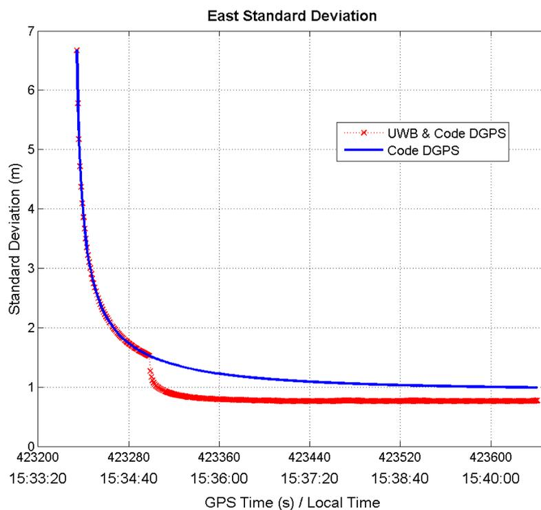
**Figure 6.17:** East position estimated standard deviation for single range UWB augmented to code DGPS, compared to code DGPS alone, for rover site #2
