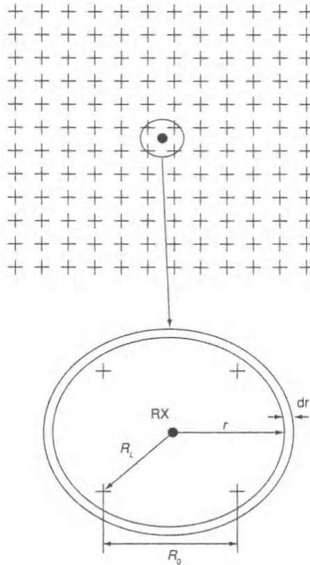
**Figure 3.8:** A dense network of UWB devices (shown as crosses) with one victim GPS receiver in the middle (shown as the black dot). This is representative of a possible UWB hotspot found in an urban area (from Nekoogar 2006).
