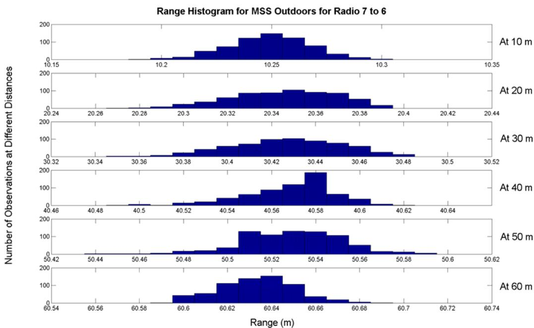
**Figure 5.23:** Range histogram of MSS radios 7 to 6 at different ranges, outdoors
