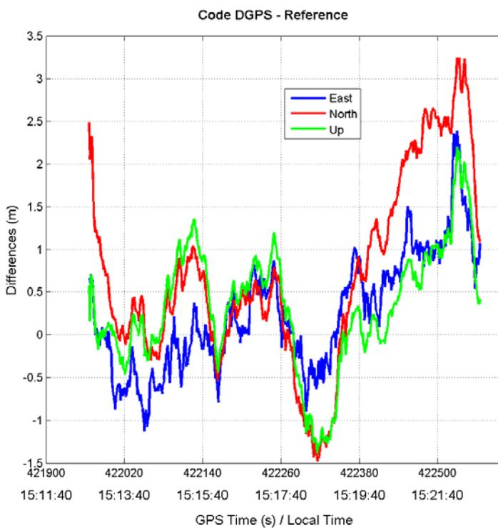
**Figure 6.7:** Difference between the code DGPS solution and GPS RTK float solution for rover site #1
