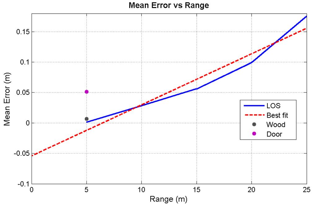
**Figure 5.4:** Mean errors for indoor TD radio measurements. Blue line results are LOS measurements, while the purple and black dots are NLOS measurements.
