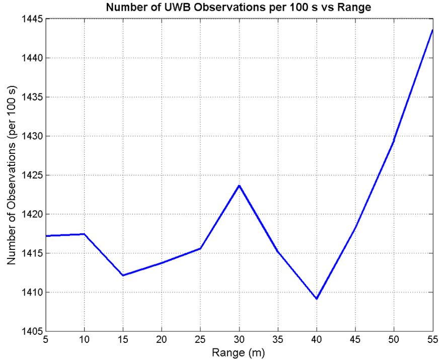
**Figure 5.7:** Number of measurements (per 100 s) versus distance for indoor MSS radios
