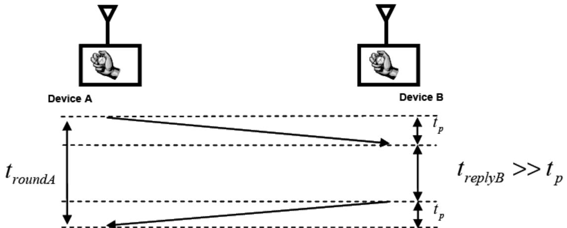
**Figure 3.6:** Two-way ranging of two devices. A range request message is sent from Device A to Device B. After a known delay ( $t_{replyB}$ ), a response is sent back from Device B to Device A
