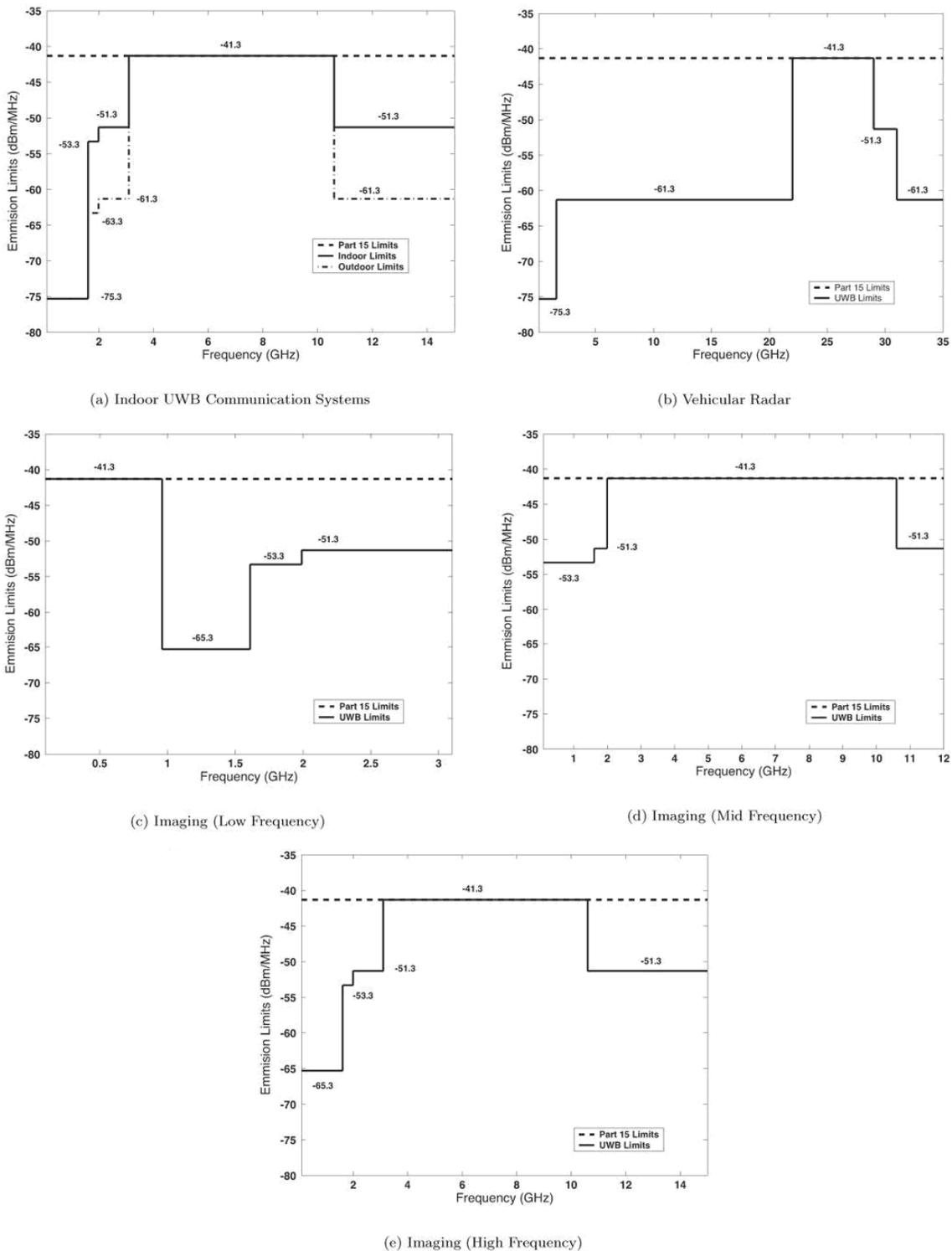
**Figure 3.7:** FCC Part 15 Spectral Mask for UWB for different applications (from FCC 2008)
