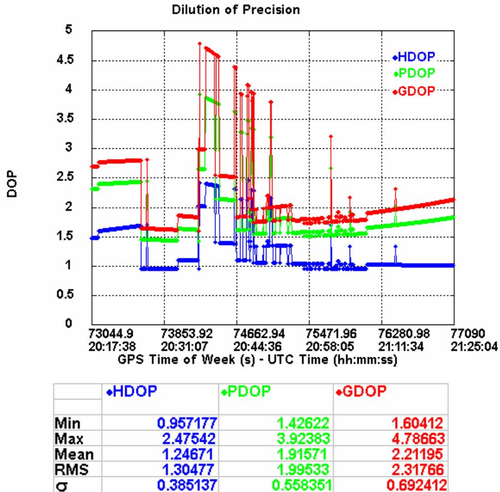
Figure 7.12: Dilution of Precision for GPS-alone solution
