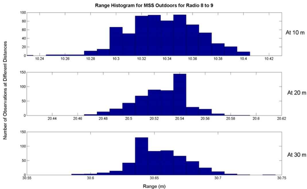
**Figure 5.24:** Range histogram of MSS radii 8 to 9 at different ranges, outdoors
