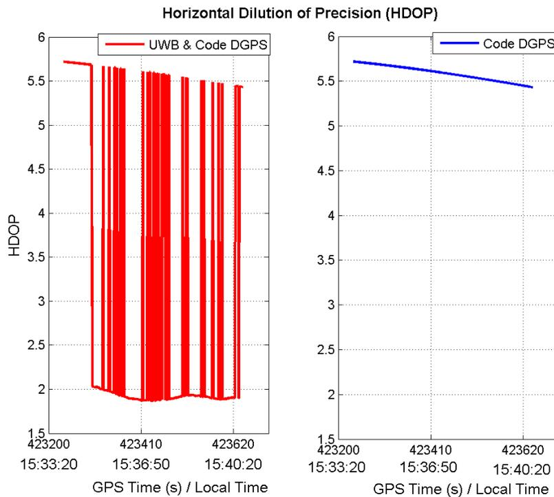
**Figure 6.20:** Horizontal DOP for single range UWB augmented to code DGPS, compared to code DGPS alone, for rover site #2
