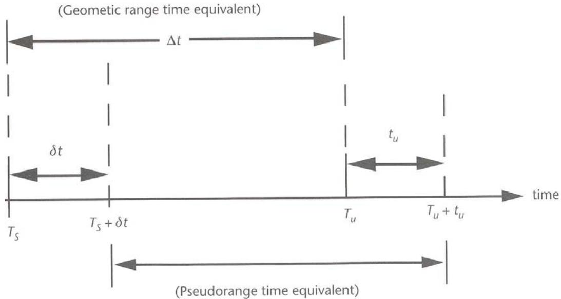
**Figure 2.1:** Two clock errors are shown to affect the pseudorange measurement in this figure with  $\delta t$  being the satellite clock error and  $t_u$  representing the receiver clock error (from Kaplan & Hegarty 2006)
