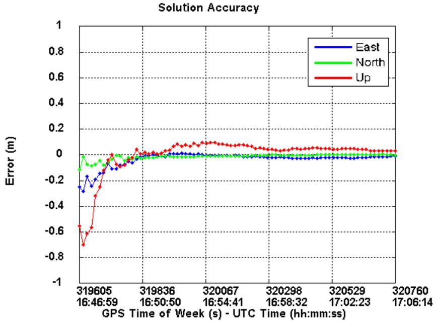
**Figure 7.2:** Position Errors for UWB-GPS solution
