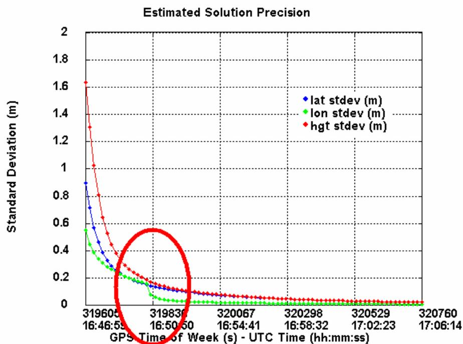
Figure 7.4: Standard deviation for UWB-GPS solution. Red circle represents the time when UWB is introduced into the GPS measurements.
