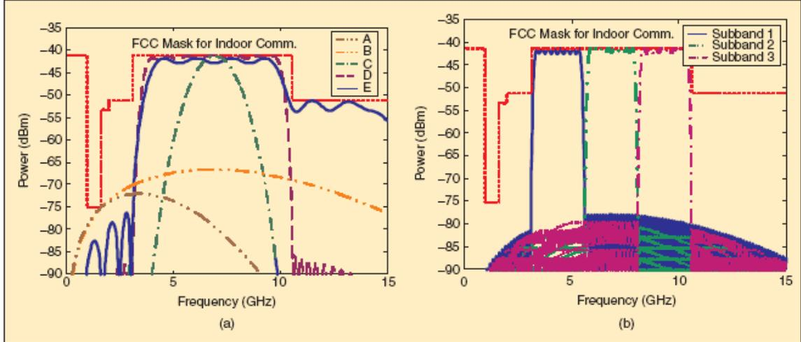
▲ 15. (a) Baseband pulse shapers and the FCC mask for indoor communications. A—Gaussian monocycle with  $T_p = 0.37$  ns; B—Gaussian monocycle with  $T_p = 0.19$  ns; C—a pulse shaper in [98]; D&E—pulse shapers in [99]; (b) Multiband UWB using baseband pulse shapers.
