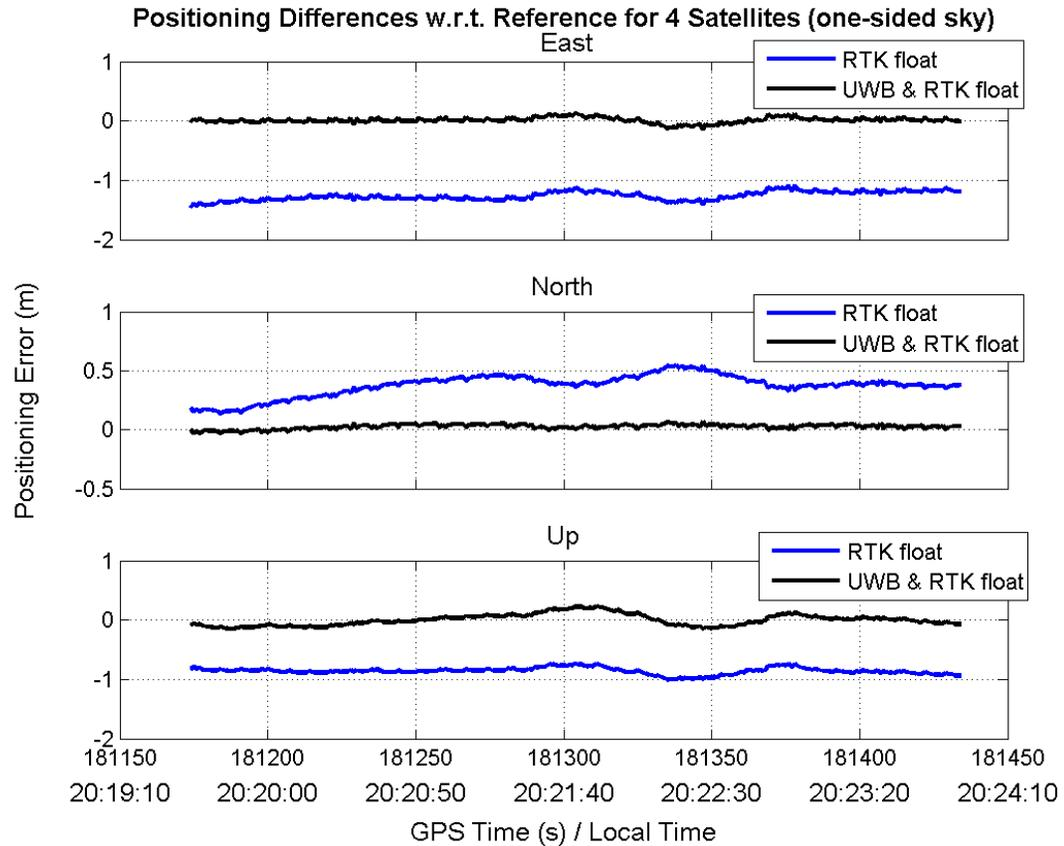
**Figure 7.29:** Positioning differences between the reference solution and RTK float with and without UWB augmentation for the “bad” signal case
