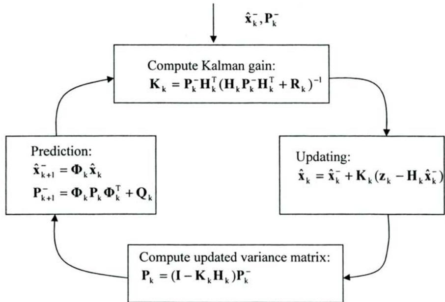
**Figure 4.1:** Standard Kalman filter algorithm (from Gao & Sideris 2005)
