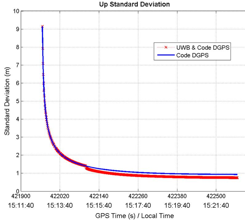
**Figure 6.14:** Up standard position for single range UWB augmented to code DGPS, compared to code DGPS alone, for rover site #1
