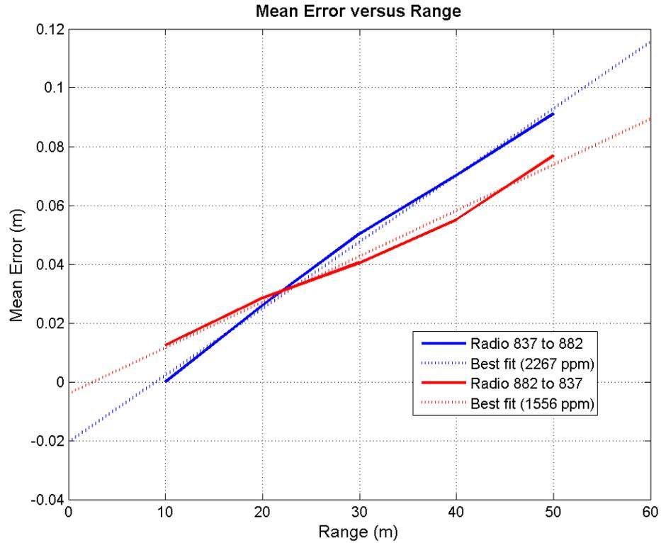
**Figure 5.18:** Mean error for two combinations of TD UWB radios, outdoors
