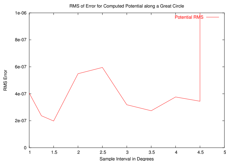
Figure 5-4: Without a priori information, arbitrary weighting or Tikhonov regularization, subsurface masses at a fixed depth can be acceptably well resolved providing the surface sampling interval is less than the subsurface interval.
