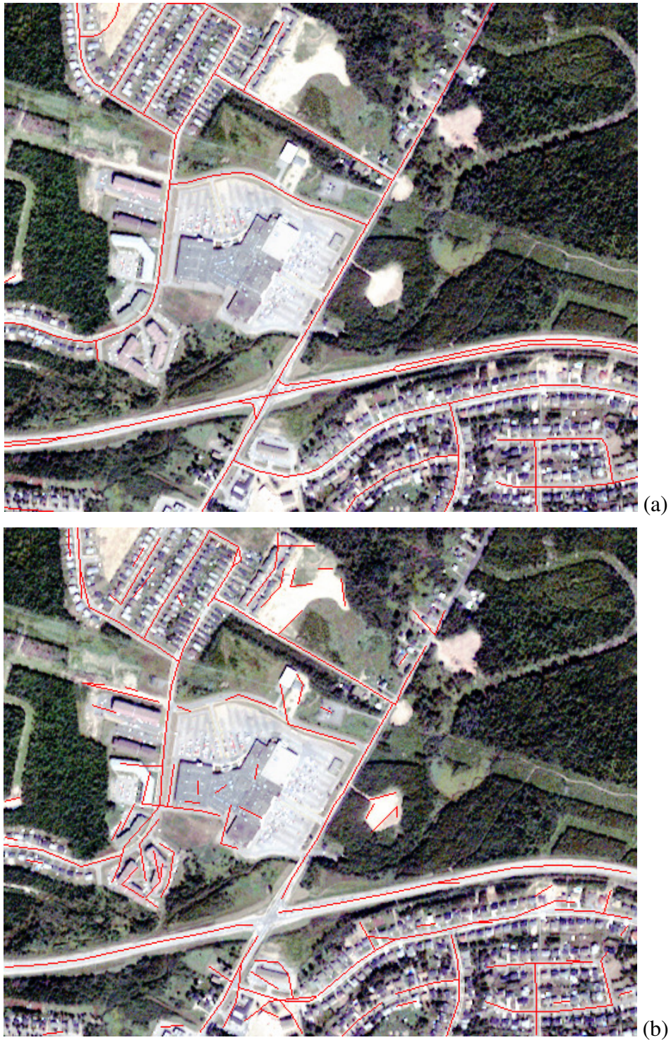
Figure 6.1 Evaluation of automated road extraction: (a) the RGB composite of the source image overlaid with the reference roads (red lines); (b) the extracted roads (red lines)
