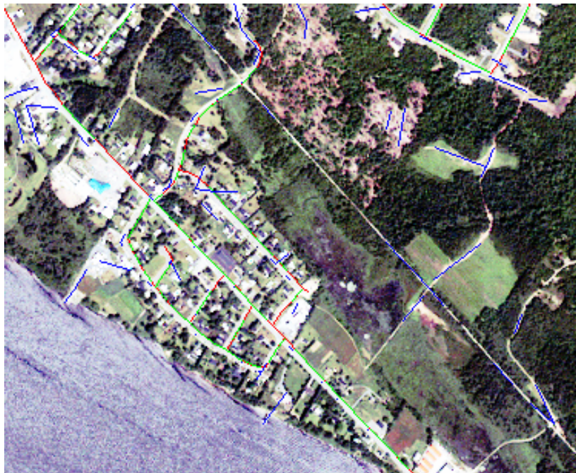
Figure 6.5 Evaluation results for the image Ikonos MS 1: Green – correct extraction, red – missed roads, blue – false extraction
