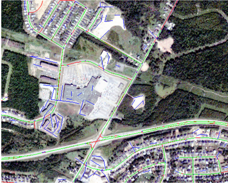
Figure 6.4 Evaluation results for the extracted road network in Figure 6.1 (b): Green – correct extraction, red – missed roads, blue – false extraction
