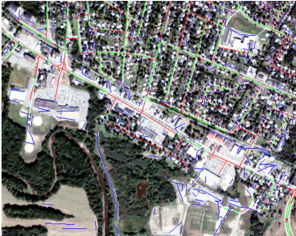
Figure 6.9 Evaluation results for the image Quickbird MS 2: Green – correct extraction, red – missed roads, blue – false extraction
