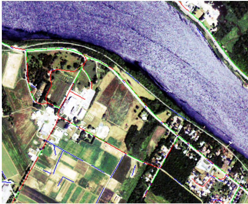
Figure 6.6 Evaluation results for the image Ikonos MS 2: Green – correct extraction, red – missed roads, blue – false extraction
