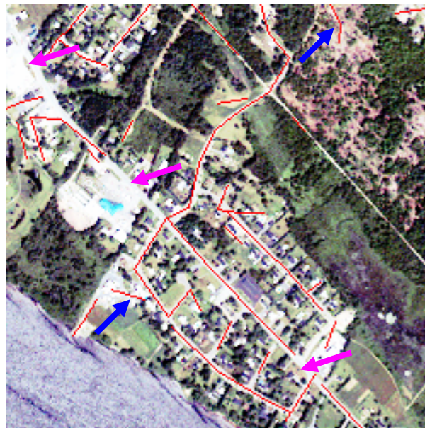
Figure 5.5 Road network formation based on the extracted road centerline segments from the Ikonos MS test image presented in Figure 2.1.
