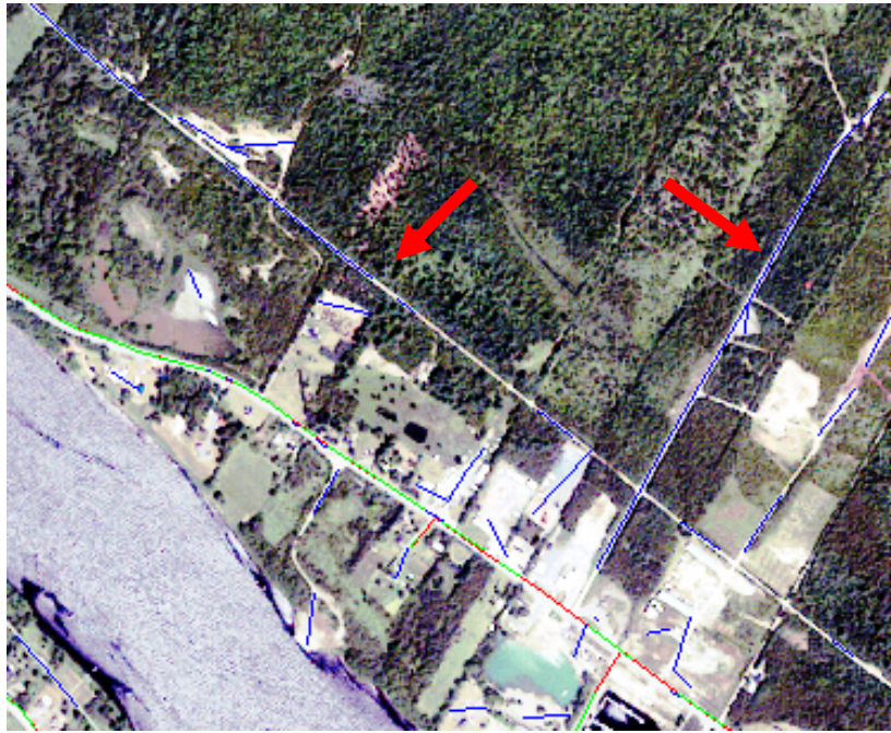
Figure 6.7 Evaluation results for the image Ikonos MS 3: Green – correct extraction, red – missed roads, blue – false extraction
