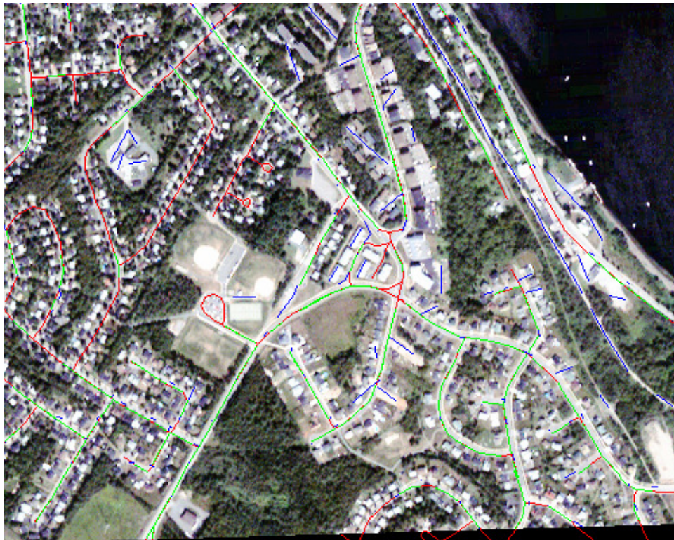
Figure 6.8 Evaluation results for the image Quickbird MS 1: Green – correct extraction, red – missed roads, blue – false extraction
