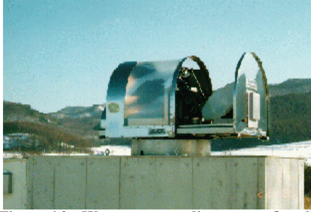
Figure 6.2: Water vapor radiometer at Onsala
