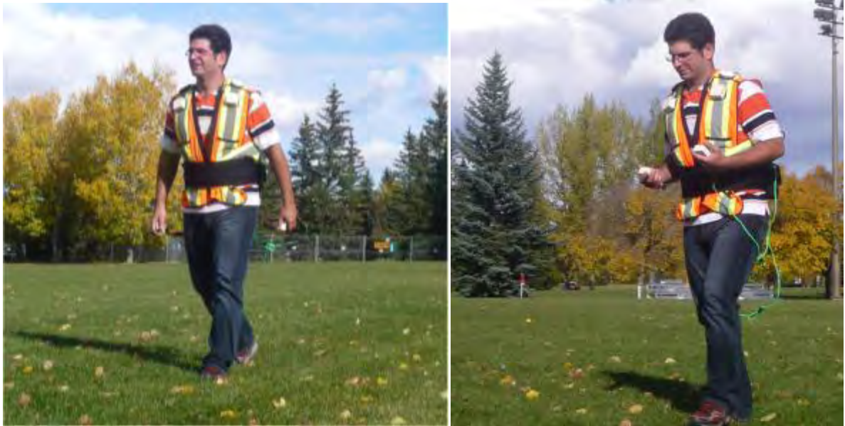
Figure 5-9: (Left ) Test subject walking with the IMUs in his swinging hands; (Right) Test subject walking with the IMUs in his texting hands.
