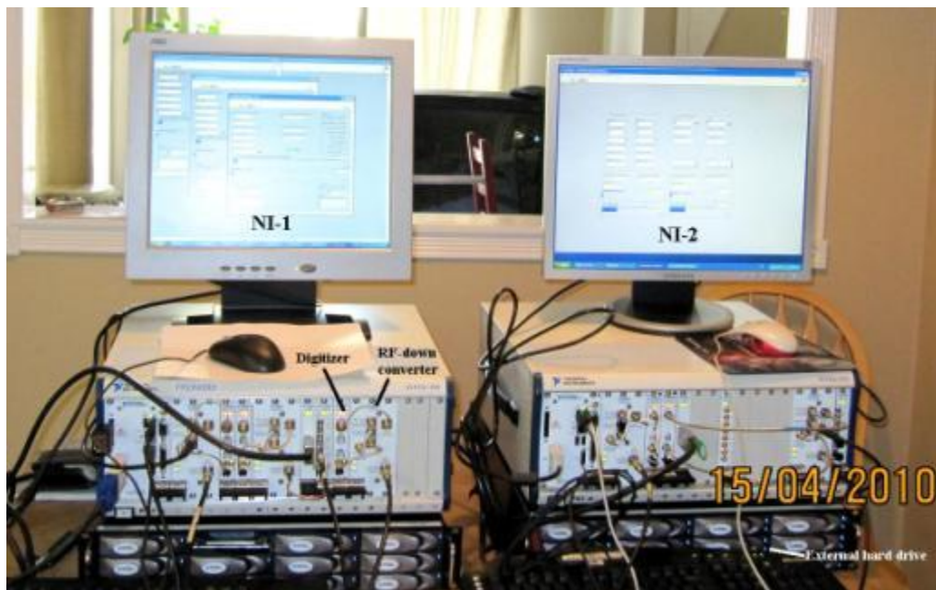
Figure 3-1: Two National Instruments signal analyzers each having multiple RF down converters and digitizers.
