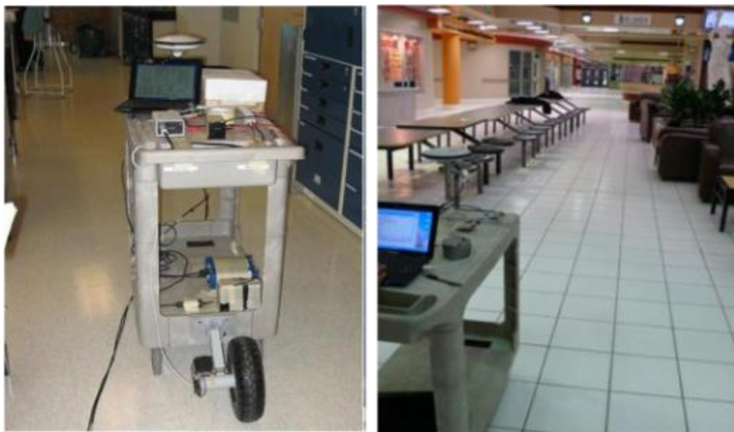
Figure 5-11: Data collection inside the NavLab (left) and McEwan Hall (right) using an instrumented cart.
