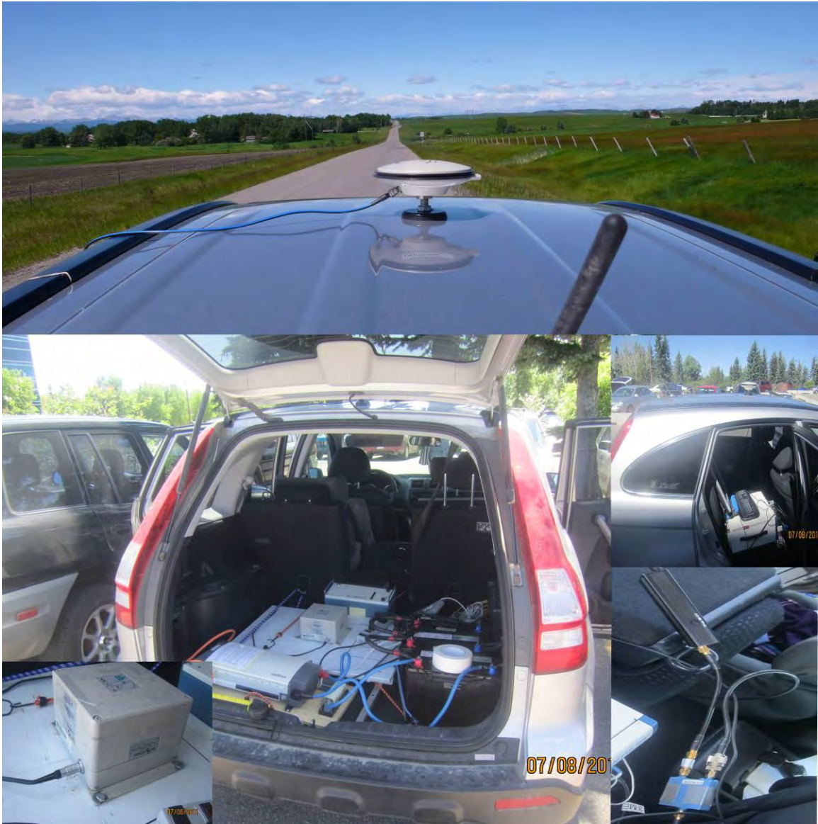
Figure 5-9: GPS antenna mounted on the SUV roof top and IMU with other equipments inside the vehicle
