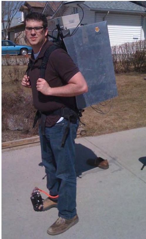
Figure 31 – Rigidly Mounted IMUs on the Foot
