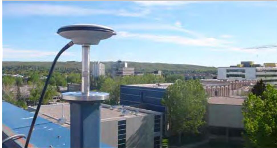
Figure 1 - Static baselines - base station
