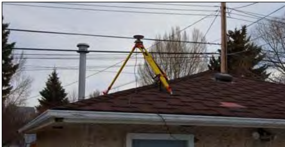
Figure 2 - Static baselines - rover station
