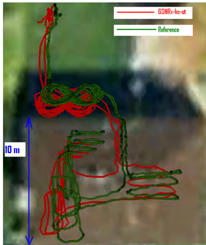
Figure 5-36 Estimated trajectories from GSNRx-hs-ut TM and the reference solution
