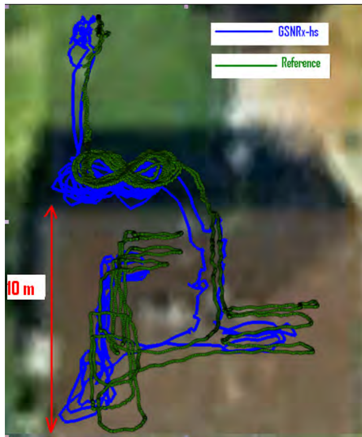
Figure 5-33 Estimated trajectories from GSNRx-hs TM and the reference solution
