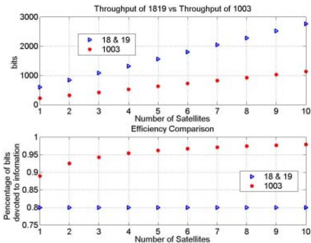
Figure 2.3: Bandwidth and efficiency comparison between RTCM 3.0 message type 1003 and RTCM 2.3 message types 18/19
