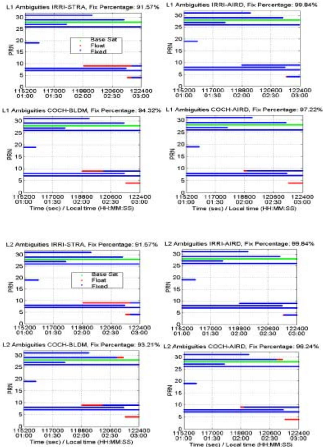
Figure 6.3: L1 & L2 ambiguity resolution status in the network
