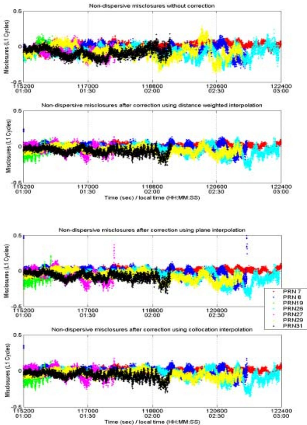
Figure 6.6: Non-dispersive “raw” and “corrected” misclosures using distance weighted, plane and collocation interpolation methods
