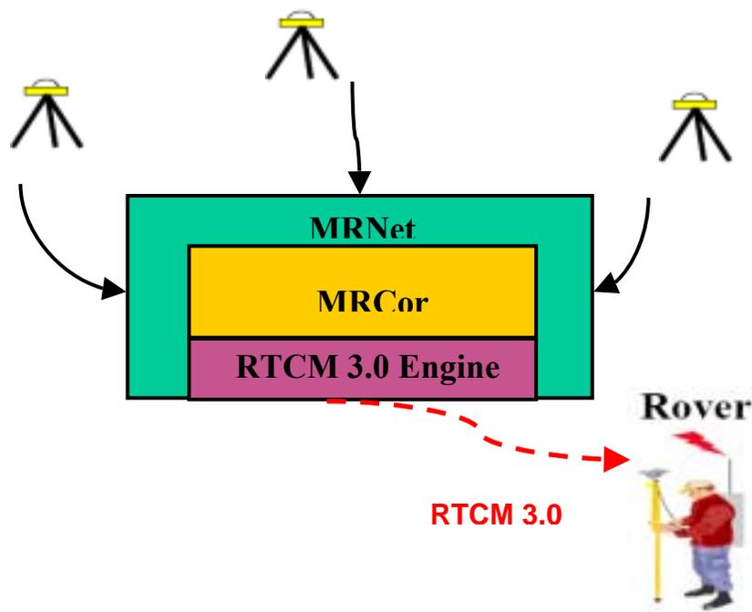
Figure 4.4: MultiRef<sup>TM</sup> RTCM 3.0 structure
