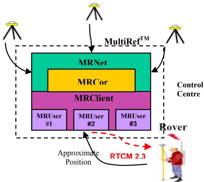
Figure 4.2: MultiRef™ option 1 structure
