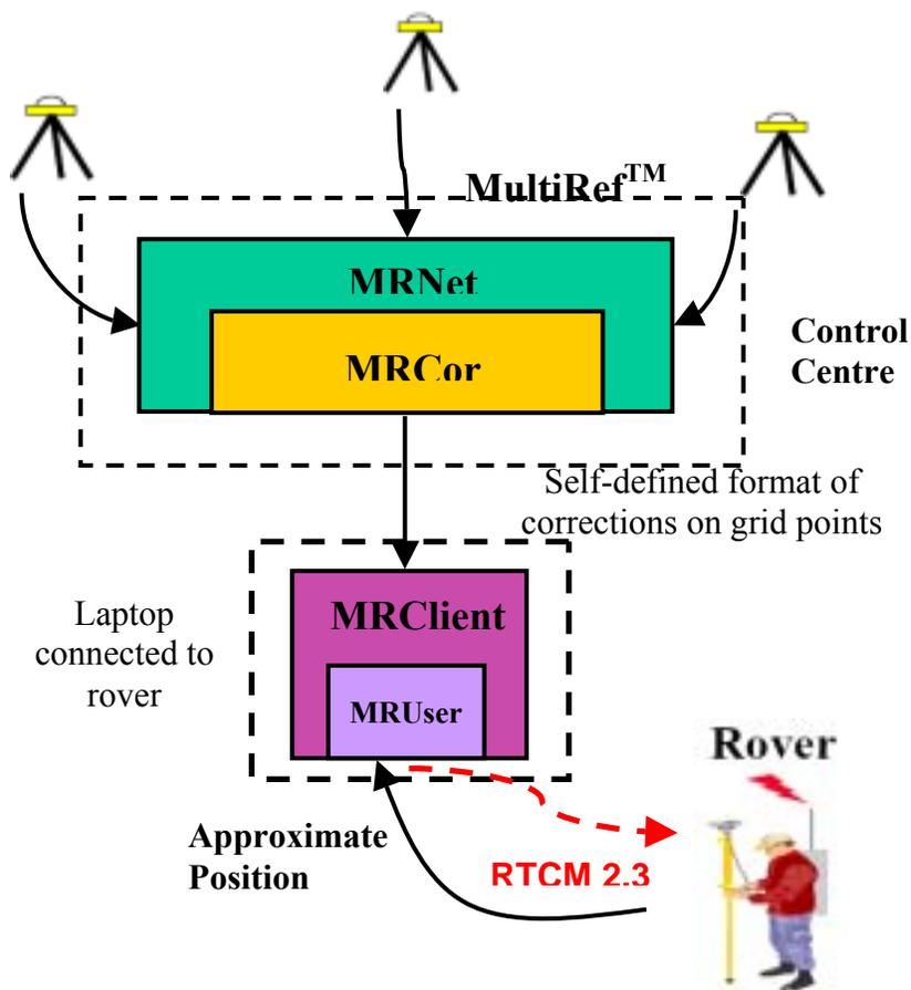
Figure 4.3: MultiRef™ option 2 structure
