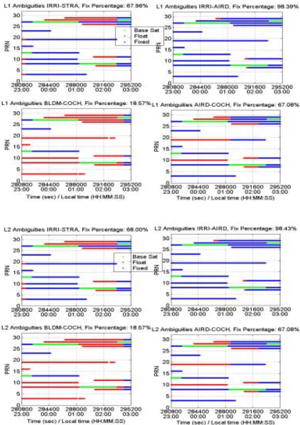
Figure 6.11: L1 &amp; L2 ambiguity resolution status in the network
