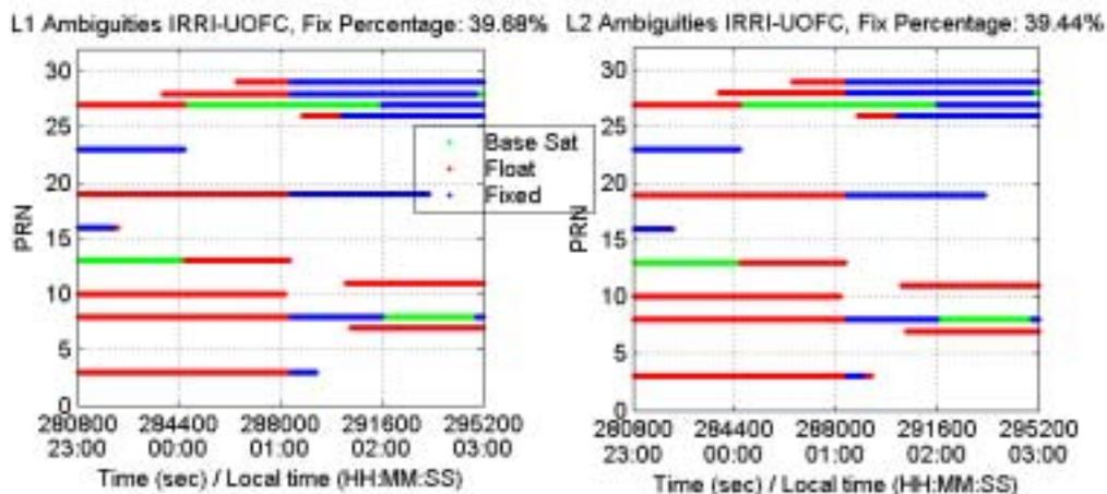
Figure 6.12: L1 and L2 ambiguity resolution between IRRI and UOFC
