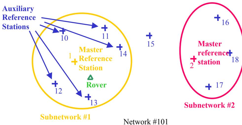
Figure 3.4: One network divided into two subnetworks
