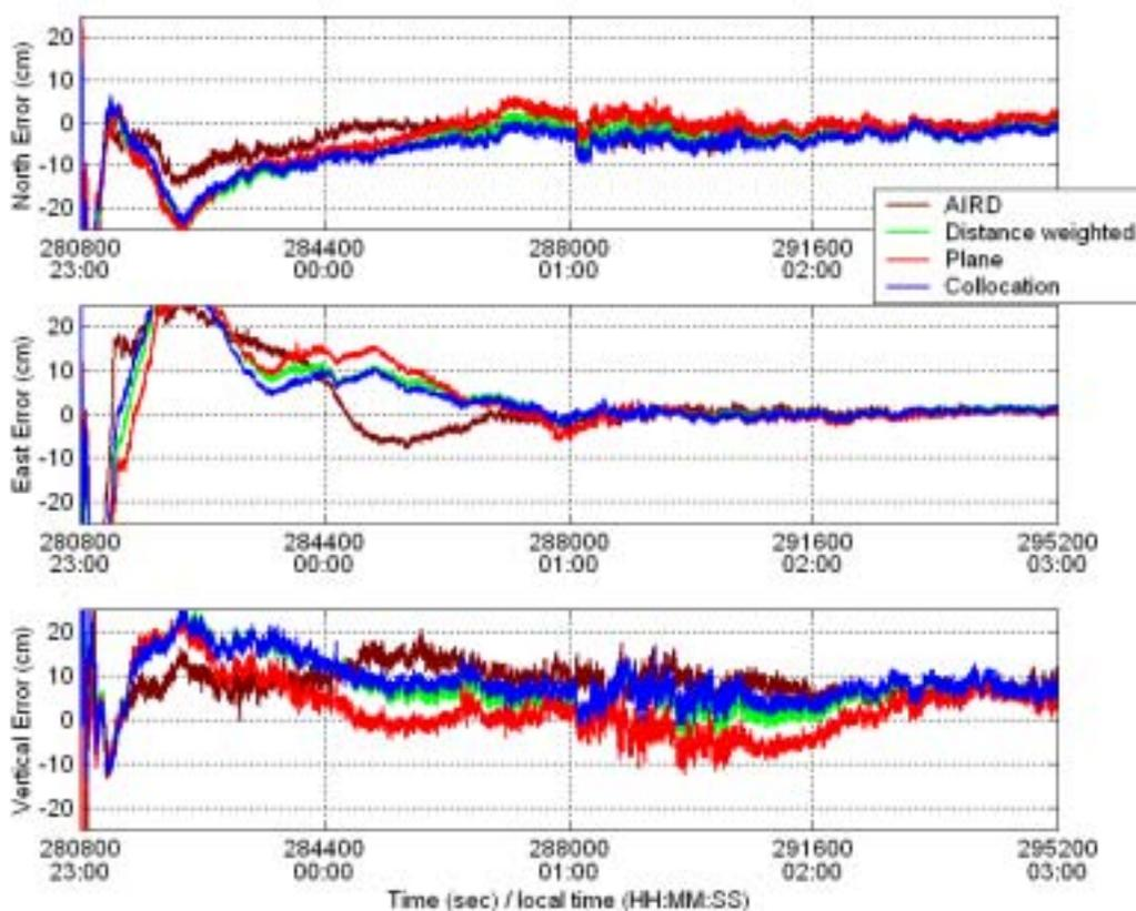
Figure 6.17: North, east and vertical position errors over time for the single reference station approach and multiple reference station approach using three interpolation methods with KAR disabled in GrafNav™
