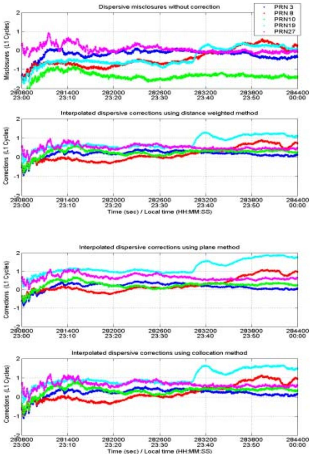
Figure 6.14: Dispersive “raw” misclosures and interpolated corrections using distance weighted, plane and collocation interpolation methods
