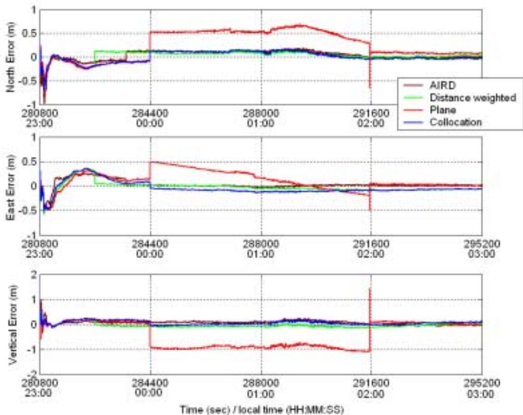
Figure 6.16: North, east and vertical position errors over time for the single reference station approach and multiple reference station approach using three interpolation methods with KAR enabled in GrafNav™
