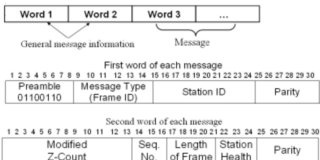
Figure 2.1: Data format of RTCM Version 2 (RTCM 2001).
