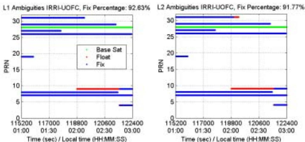
Figure 6.4: L1 and L2 ambiguities resolution between IIRI and UOFC
