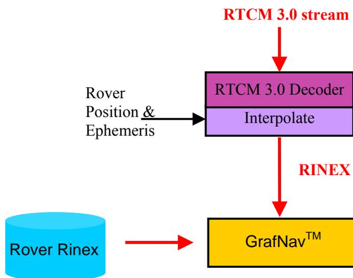
Figure 5.1: Post-mission test scheme at rover
