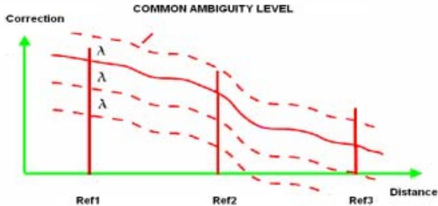
Figure 3.1: Common ambiguity level ( $\lambda$  is the wavelength of GPS signals)
