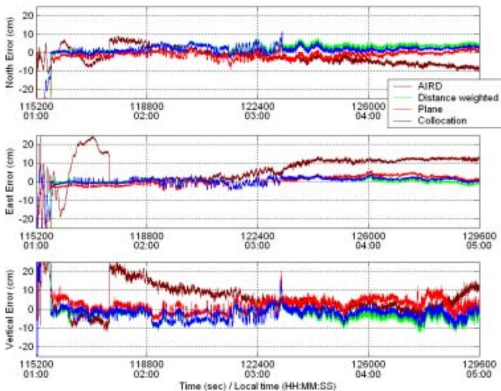
Figure 6.10: North, east and vertical position errors over time for the single reference station and multiple reference station approaches using three interpolation methods.
