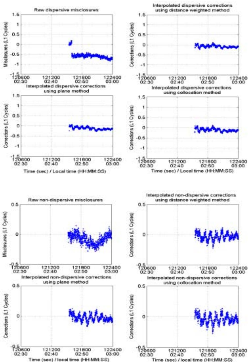
Figure 6.9: PRN4 – PRN 28 (base) “raw” misclosures on baseline IRRI-UOFC and interpolated corrections
