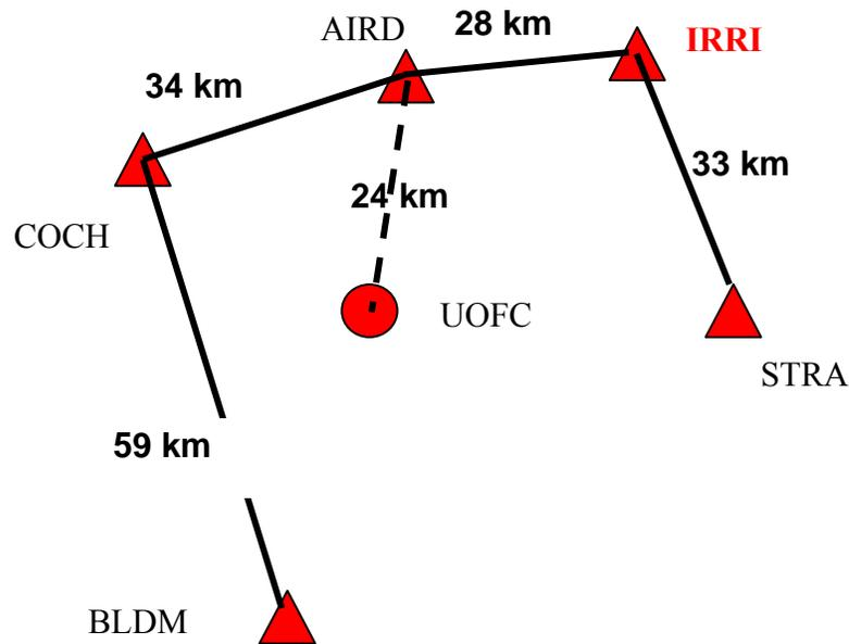
Figure 6.2: Network configuration (the master station is shown in red.)
