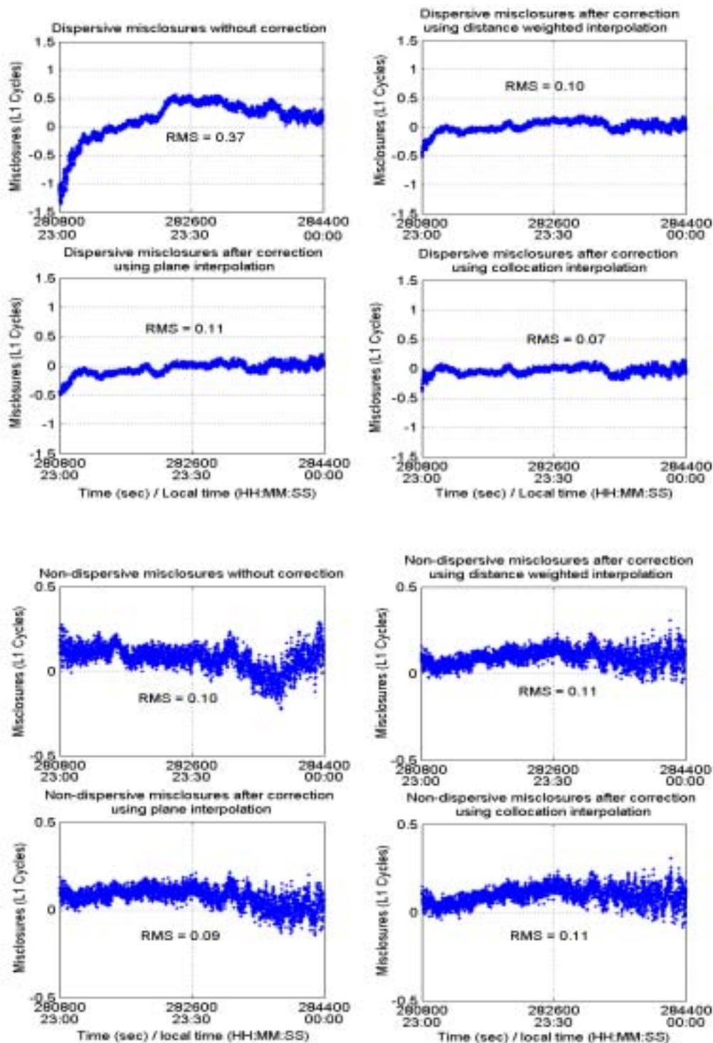
Figure 6.13: PRN 23 – PRN 13 (base) dispersive and non-dispersive “raw” and “corrected” misclosures using distance weighted, plane and collocation interpolation methods
