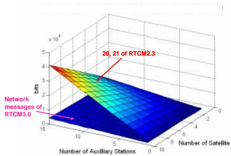
Figure 3.7: Throughput analysis of RTCM 3.0 GNSS network corrections and phase and pseudorange corrections of RTCM 2.3
