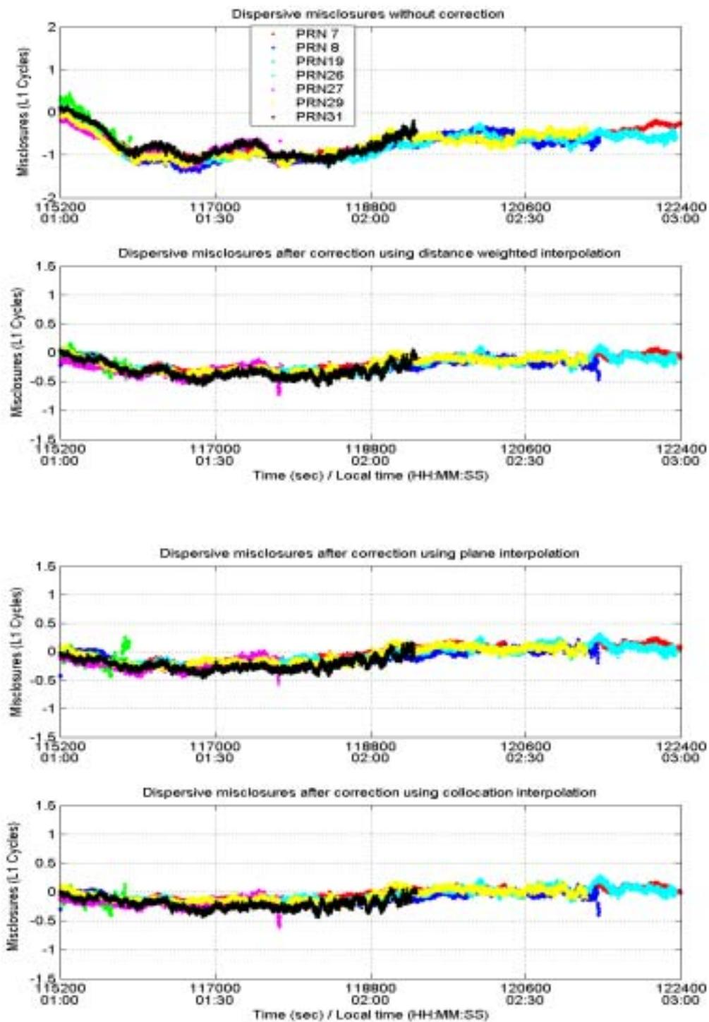
Figure 6.5: Dispersive “raw” and “corrected” misclosures using distance weighted, plane and collocation interpolation methods
