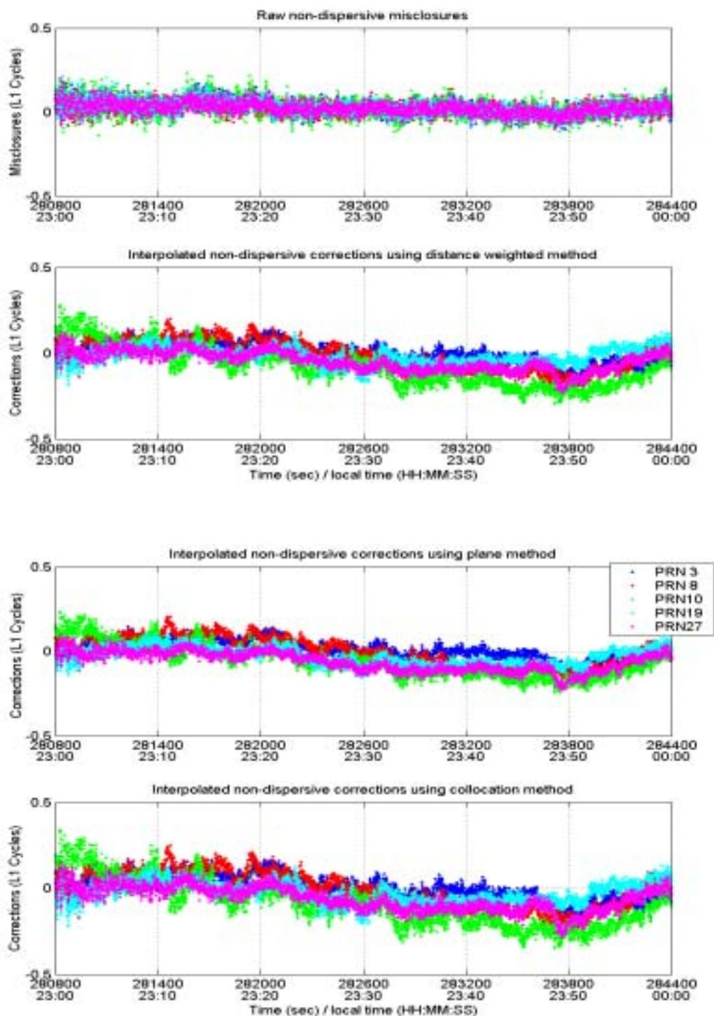
Figure 6.15: Non-dispersive “raw” misclosures and interpolated corrections using distance weighted, plane and collocation interpolation methods
