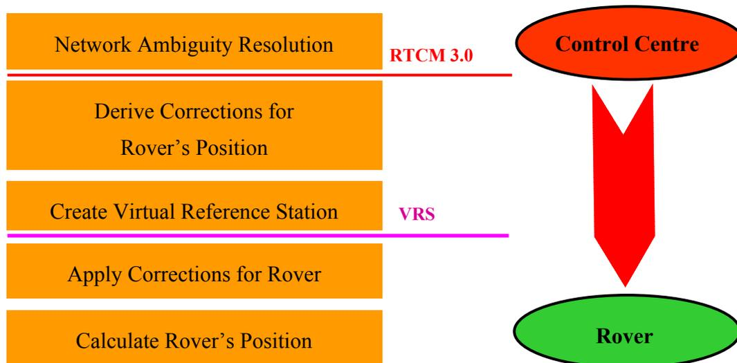
Figure 4.1: VRS and RTCM 3.0 function partitioning
