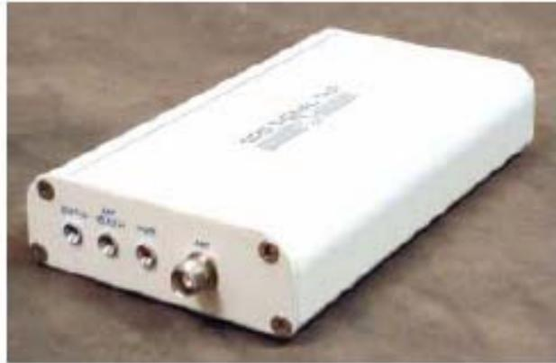
Figure 3.2: Hardware front-end “GPS Signal Tap”
