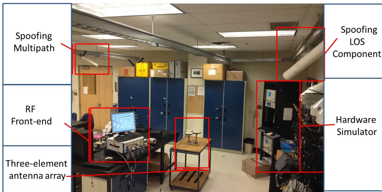
Figure 6-10: Real data collection test setup
