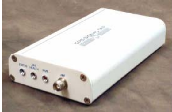
Figure 5.1: Hardware front-end “GPS Signal Tap”
