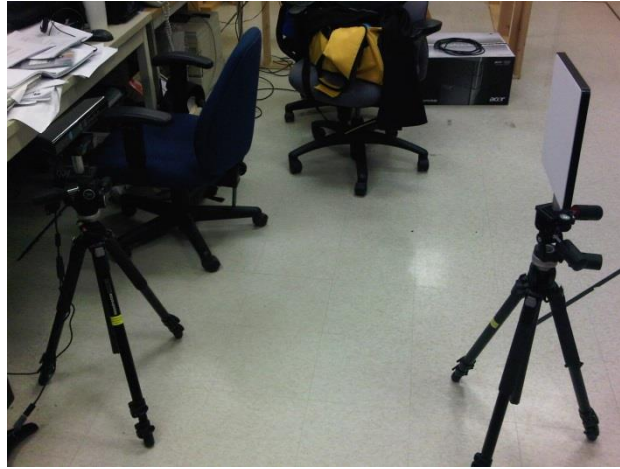
Figure 1: Data capture of a white planar Spectralon target using the Microsoft Kinect
