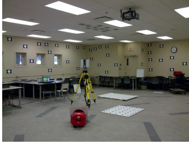
Figure 17. TLS user self-calibration at the University of Calgary.
