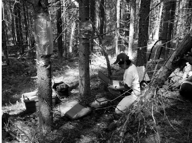
Figure 3.2: Installation of TDP sensors in a set of coniferous trees, site Conifer-4.
