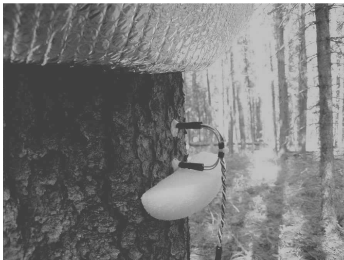
Figure 6.2: Same coniferous tree with the isolation material (upper part of the picture) ready to cover the sensors.
