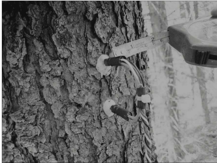
Figure 6.1: Thermal Dissipation Sensors (TDP's) installed in a coniferous tree.
