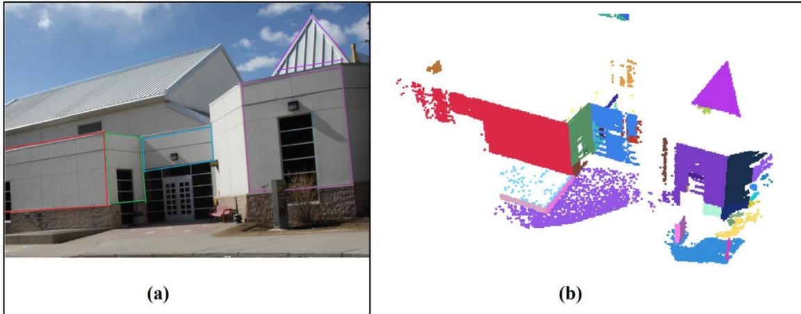
Figure 2.7. Planar features in photogrammetric data (a) and TLS scan (b)
