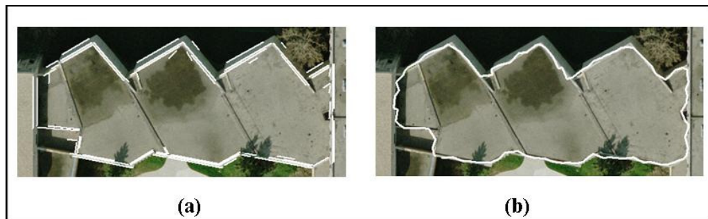
Figure 4.12: Automated linear feature extraction from perspective imagery (a), and segmented roof boundaries from the raw LiDAR data (b).
