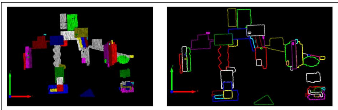
Figure 4.11: The results from segmentation of the building hypotheses (a), and the initial building-primitive boundaries (b), for the area of interest shown in Figure 4.4.
