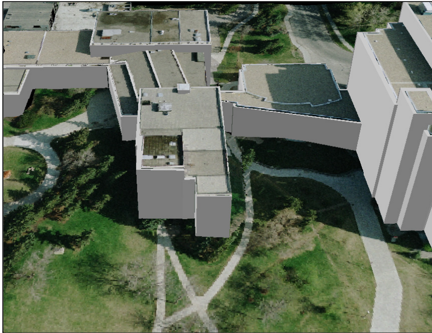
Figure 5.21: The refined DSM obtained by adding the DBM to the ground TIN.
