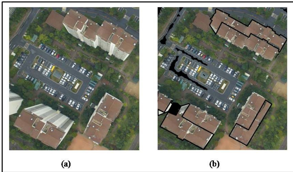
Figure 2.3: Perspective image (a) and corresponding orthophoto, with double mapped areas outlined in black (b).
