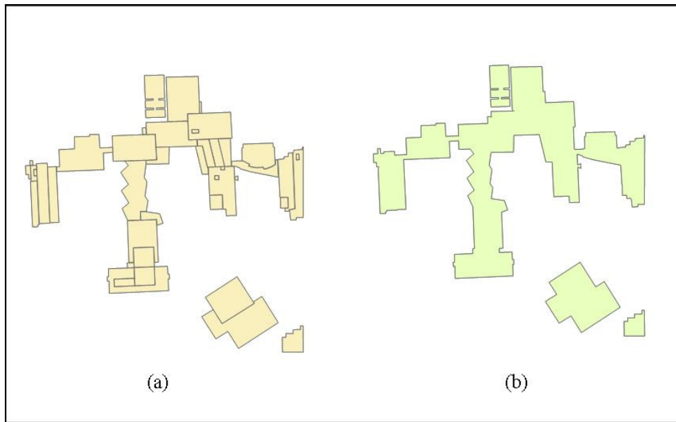
Figure 4.35: The building rooftop polygons (a) and the aggregated building footprints (b).
