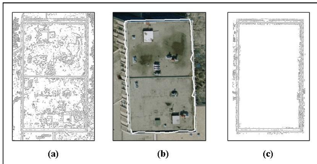
Figure 4.18: Detected edge pixels for a given building-primitive (a), the projected LiDAR building-primitive boundary (b), and the resulting edge pixels located within a LiDAR buffer area (c).
