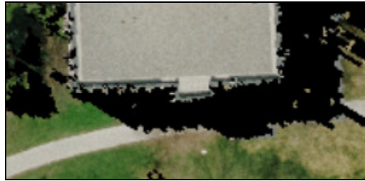
Figure 2.13: Scissoring effects in orthophoto due to original LiDAR-derived DSM.
