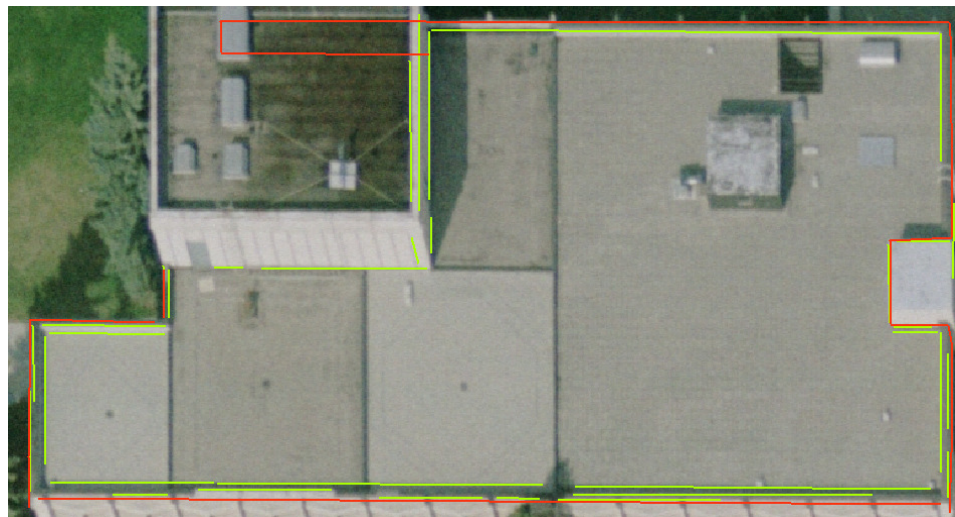
Figure 4.28: The display of detected lines from multiple images - red lines from previous image, green from current.
