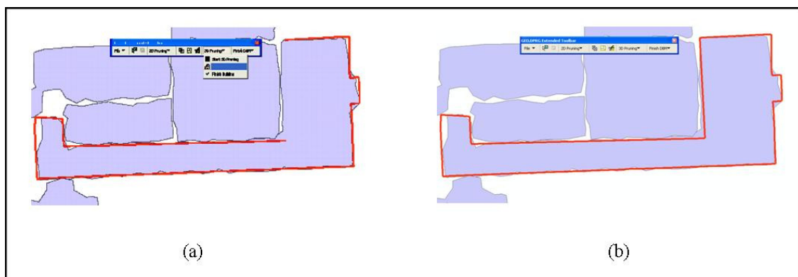
Figure 4.33: Use of the LiDAR boundary for manual editing in 3D, where a) and b) represent the boundary outline before and after editing.
