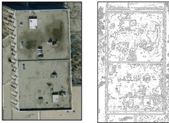
Figure 4.15: Sample output from edge detection algorithm, showing the large quantity of edges that are detected for the given building-primitive.
