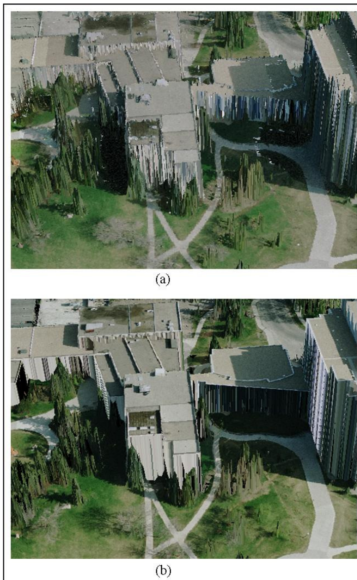
Figure 5.20: The 3D models created using the original LiDAR derived DSM (a), the DSM obtained by adding the DBM to the original DSM (b).
