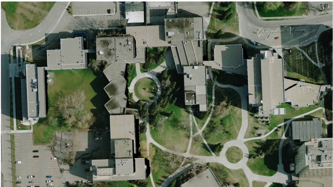
Figure 6.15: A true orthophoto produced using the enhanced DSM and the imagery involved.
