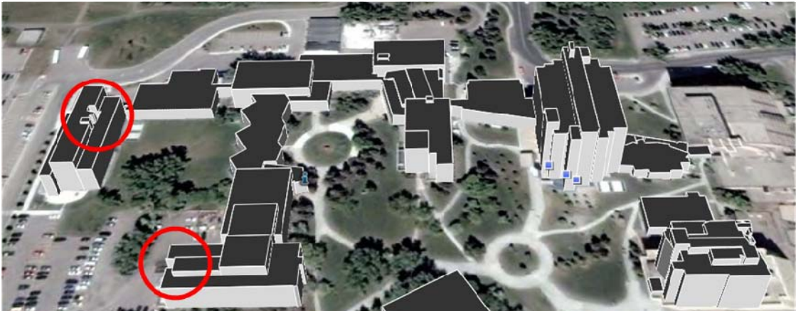
Figure 6.11: Initial DBM (in KML format) produced through the automated building reconstruction process.
