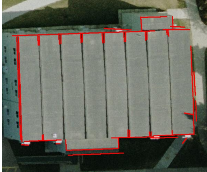
Figure 5.14: Matched 3D lines for the straight line segments in Figure 5.12(a) and (b).
