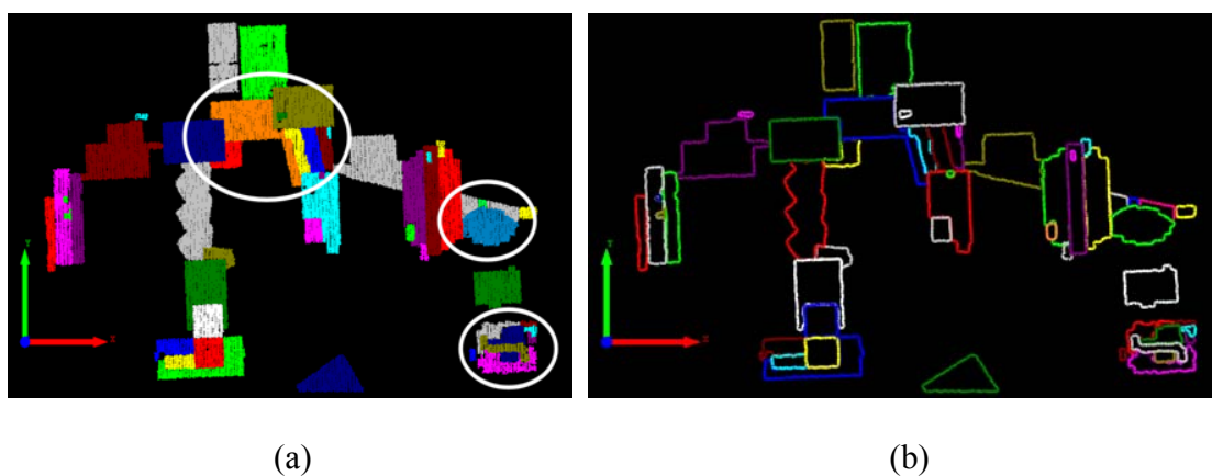
Figure 6.5: Clustered building primitives (a), and the initial boundaries of the building primitives (b).
