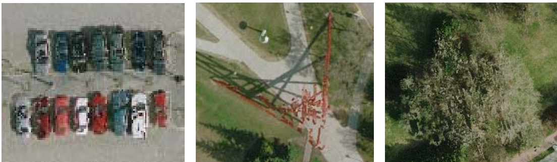
Figure 3.22: Low quality of the produced true orthophoto around small features (e.g., cars, sculptures, and trees) due to the incompleteness of the DSM.
