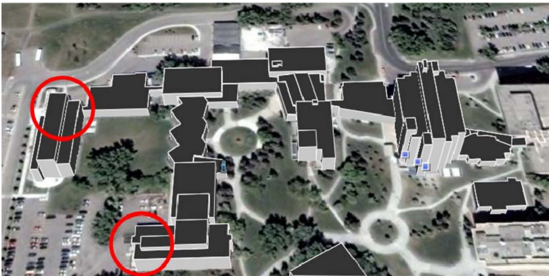
Figure 6.13: Final DBM (in KML format) after manual editing of the initial DBM, which is produced through the automated process.
