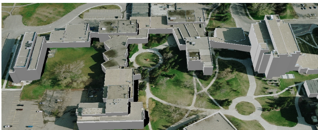
Figure 6.16: A 3D visualization produced by draping the true orthophoto over the enhanced DSM.
