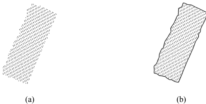
Figure 4.24: Boundary detection: clustered points from attribute space (a), and detected boundary (b).
