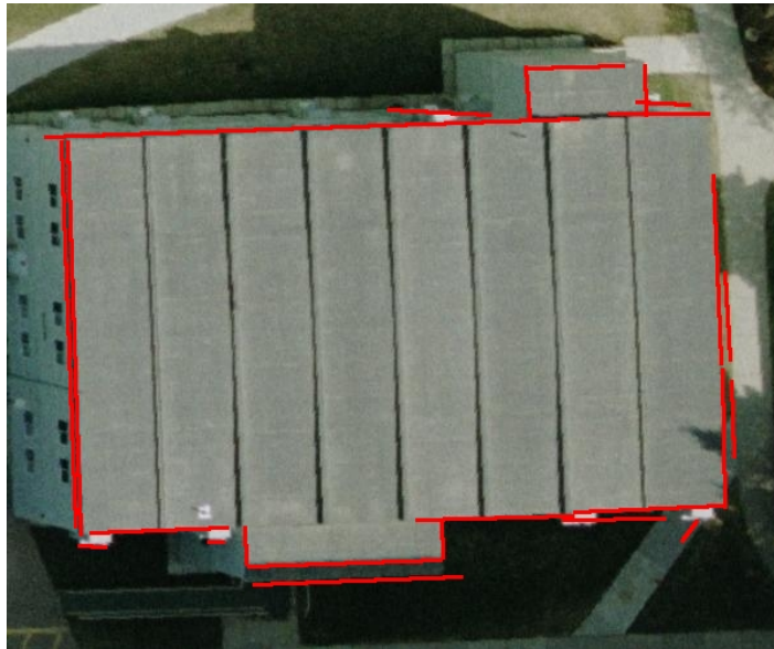
Figure 5.16: Filtered matched 3D lines which are obtained after the filtering process is applied to the matched 3D lines in Figure 5.14.
