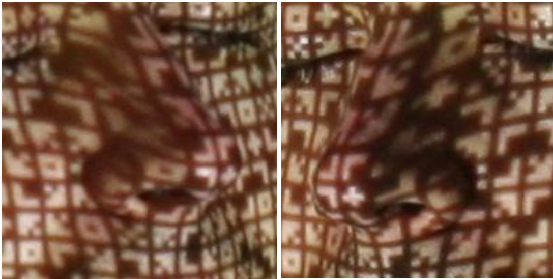
Figure 3.18: Significant differences of relief displacement between images with a large baseline.
