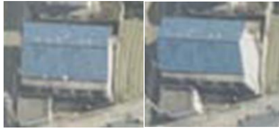
Figure 3.5: Significant differences in relief displacement caused by the location of the object within the field of view of the imaging sensor (Wang et al., 2007).
