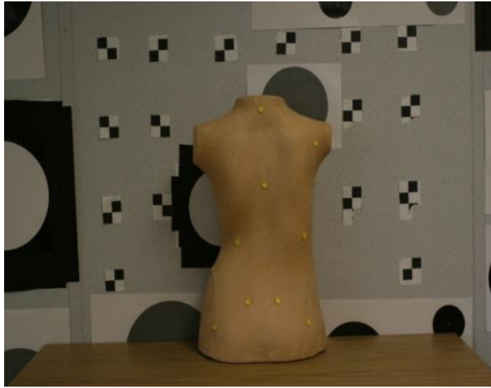
Figure 4.14: The control targets on the wall are not easily identifiable in the images without pattern projection.
