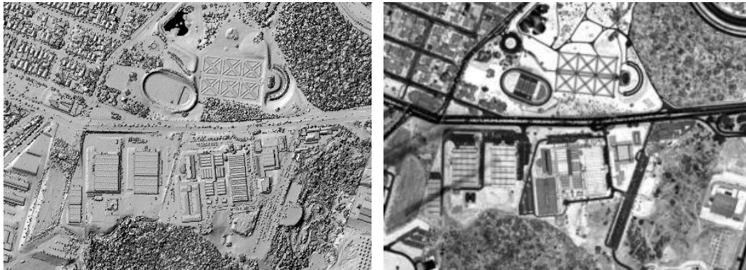
Figure 1.2: Sample LiDAR imagery: range (shaded relief) image (left) and intensity image (right).
