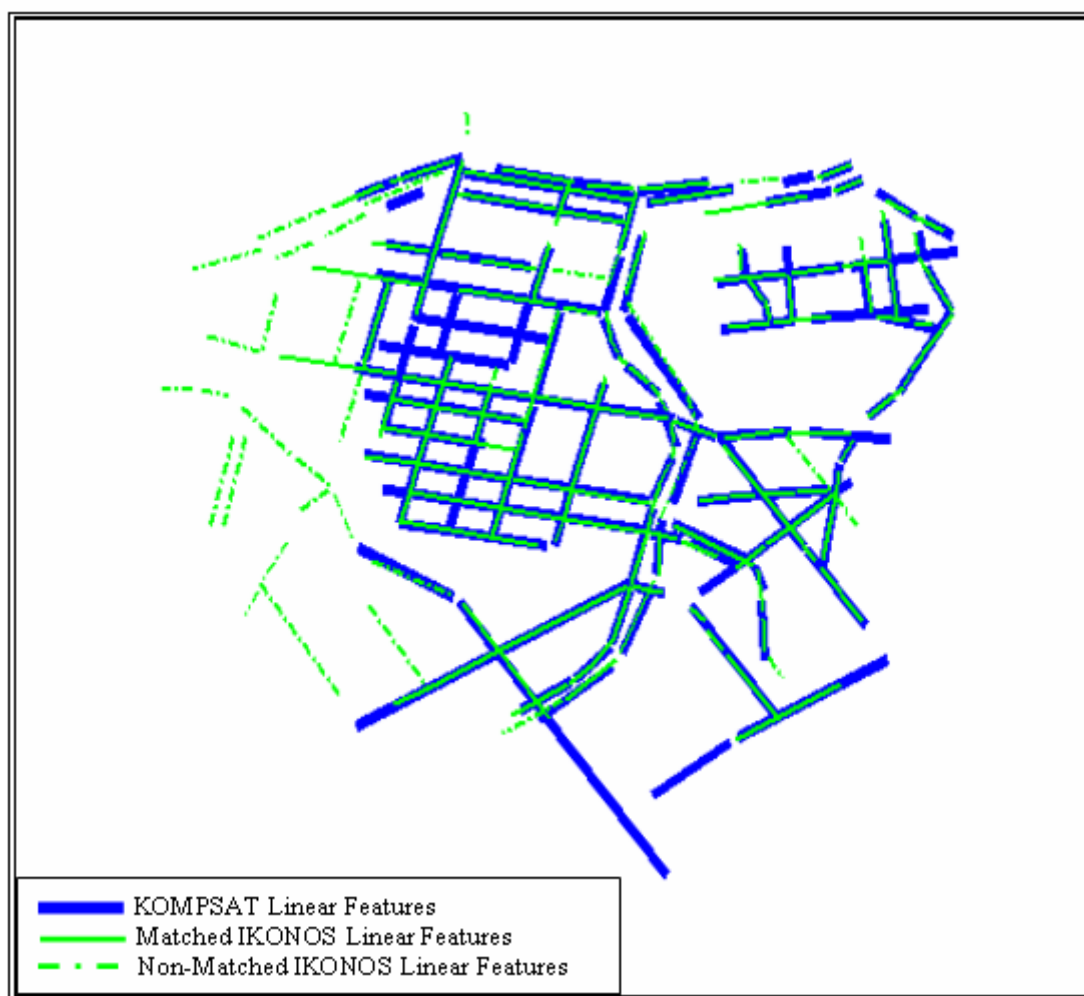
Figure 6.4: Established Correspondences between IKONOS and KOMPSAT Primitives.
