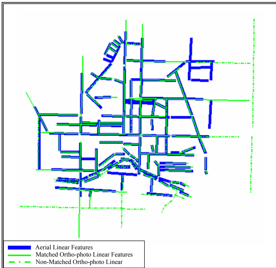
Figure 6.7: Established Correspondences between Ortho-photo 1999 and Aerial 1956 Primitives.
