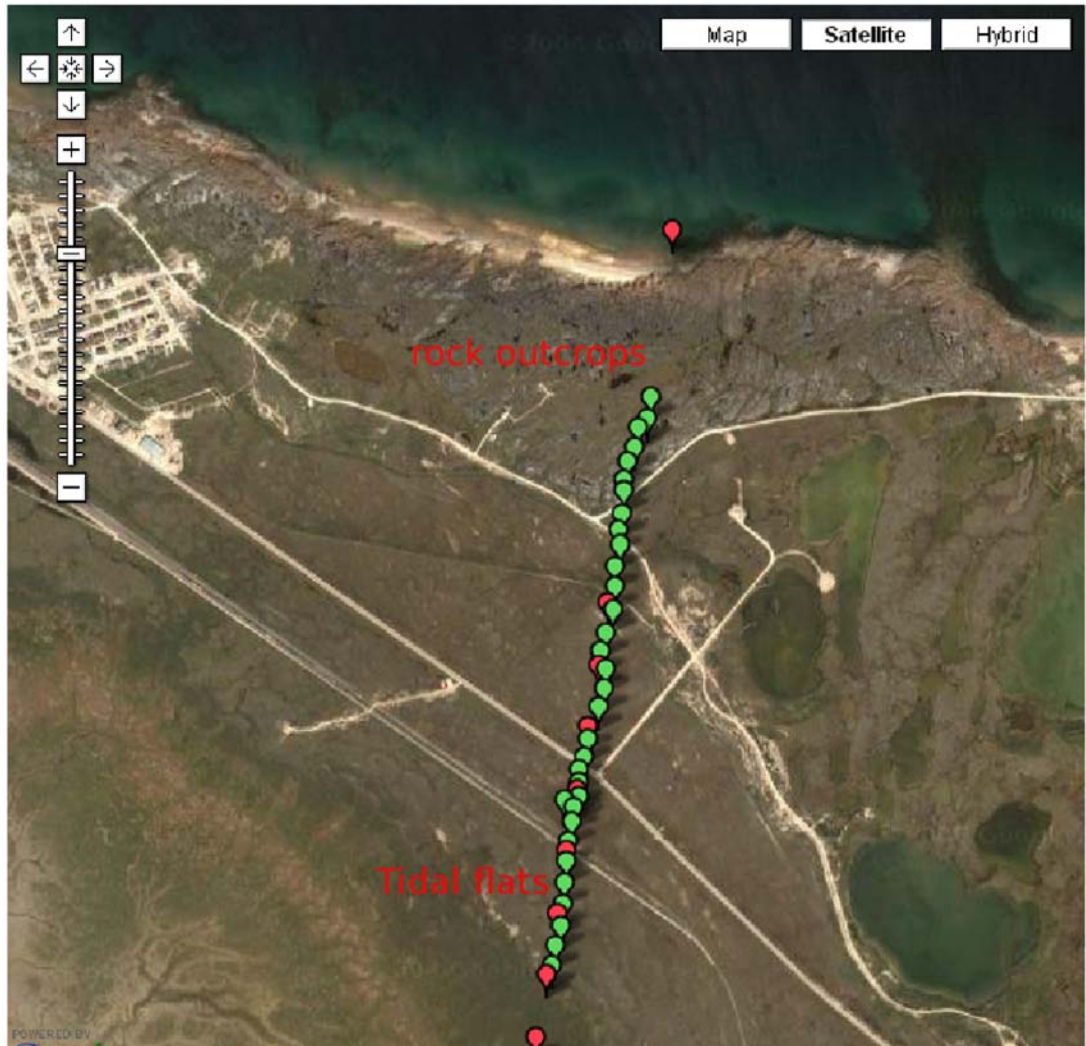
Figure 6.1: ICESat footprints (in red) and leveling survey points (in green) along the TIDAL FLATS track in Churchill, Manitoba, Hudson Bay. ©Google Maps.
