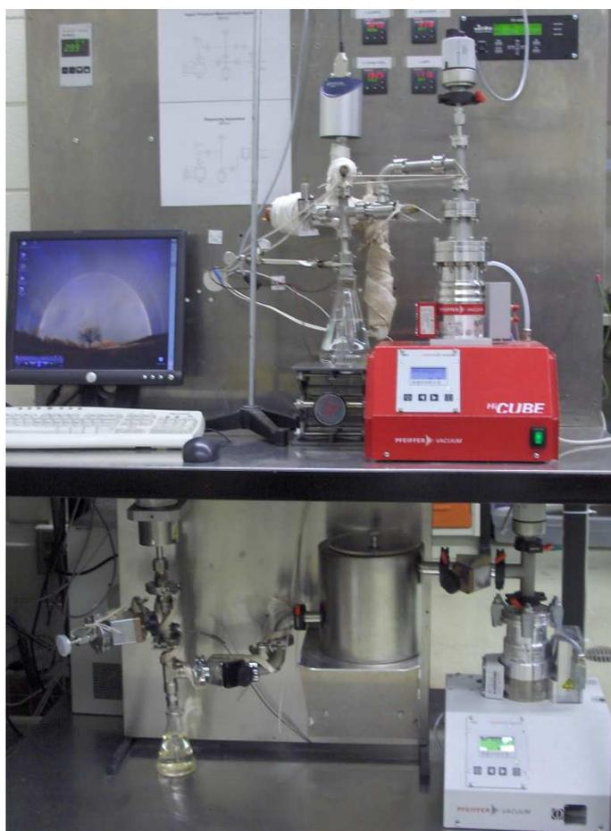
**Figure B.5** High Vacuum Vapour Pressure Measurement system (HV-VPMS); Vapour Pressure Measurement Apparatus VPMA (above) and Degassing Apparatus DA (below)
