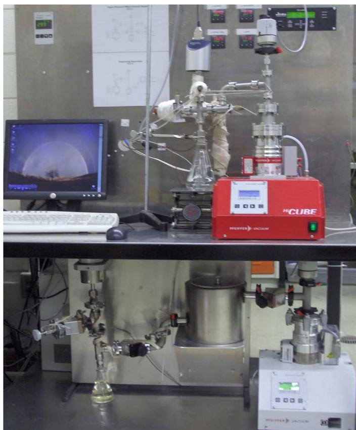
**Figure 3.16** High Vacuum Vapour Pressure Measurement system (HV-VPMS); Vapour Pressure Measurement Apparatus VPMA (above) and Degassing Apparatus DA (below).
