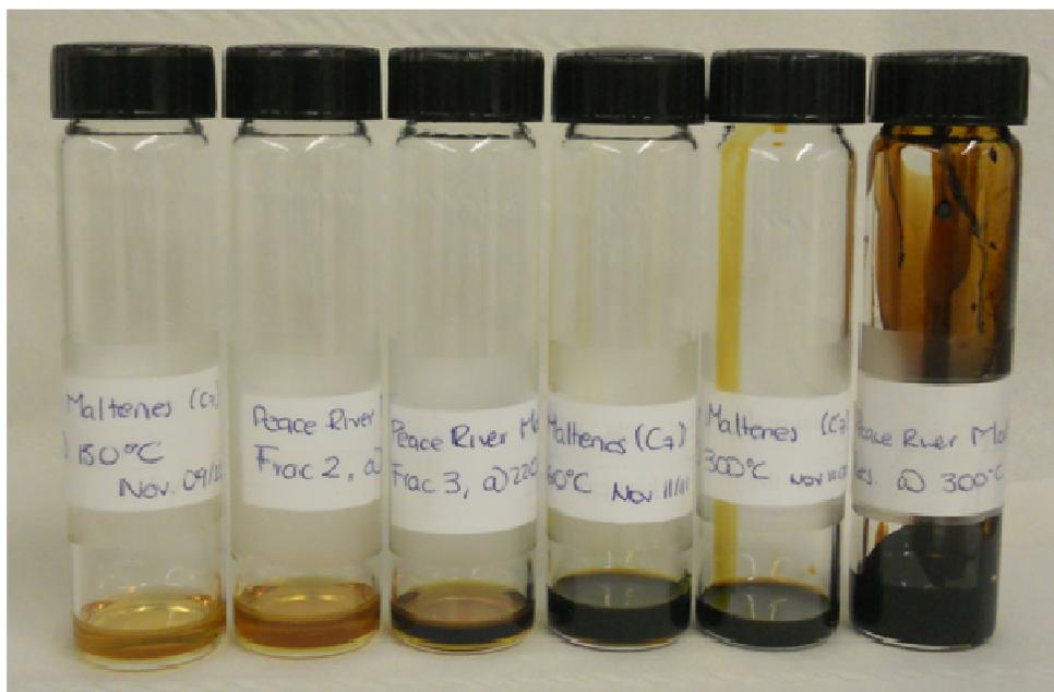
**Figure 8.24** Photograph of five the different fractions and residue of WC\_B1 maltenes deep vacuum fractionation.
