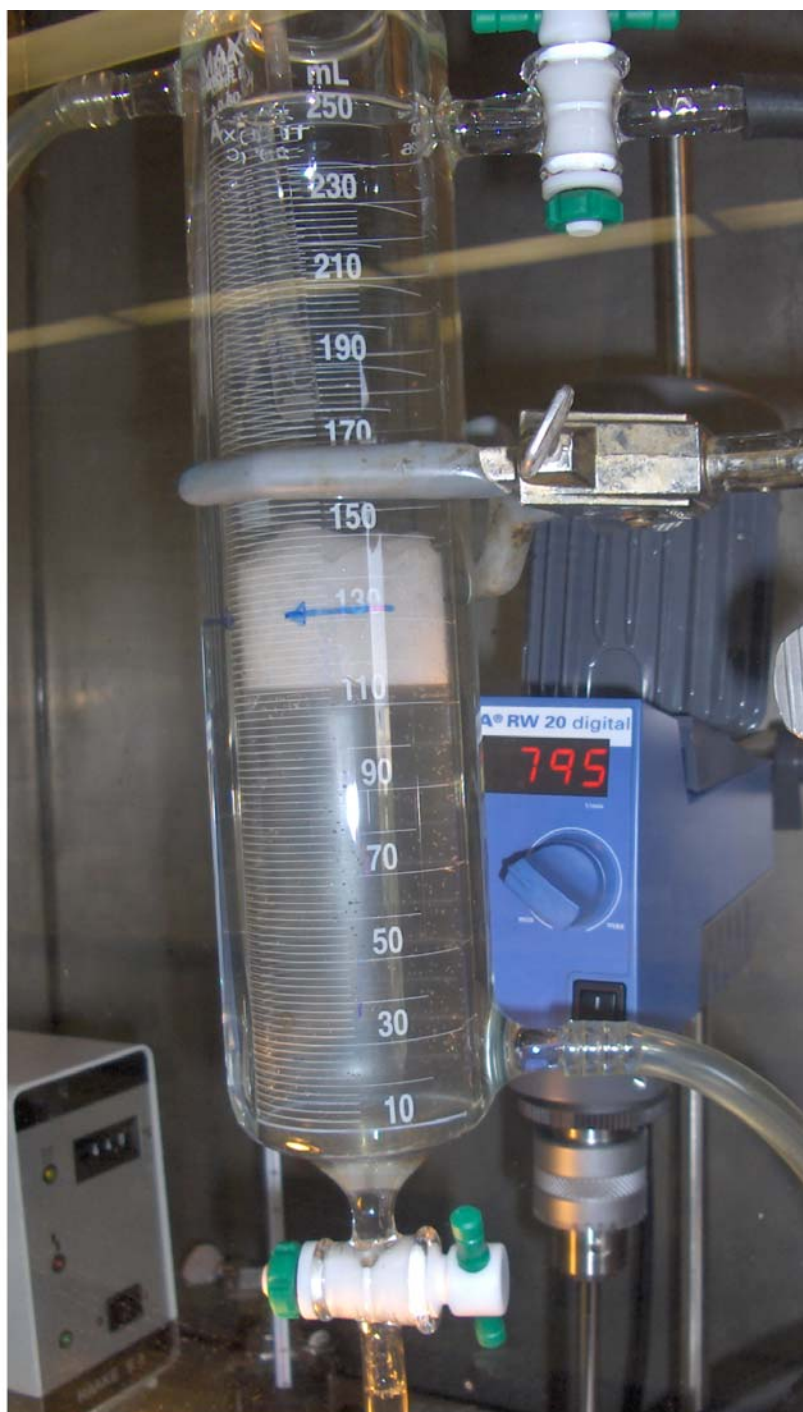
Figure 3.8 Photograph of a continuous separator experiment. Three layers are visible in the column: oil phase (top), rag layer (center) and aqueous phase (bottom).
