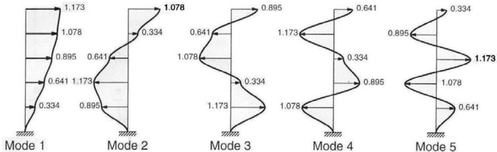
$$T_1 = 2.01s \quad T_2 = 0.68s \quad T_3 = 0.42s \quad T_4 = 0.34s \quad T_5 = 0.29s$$
