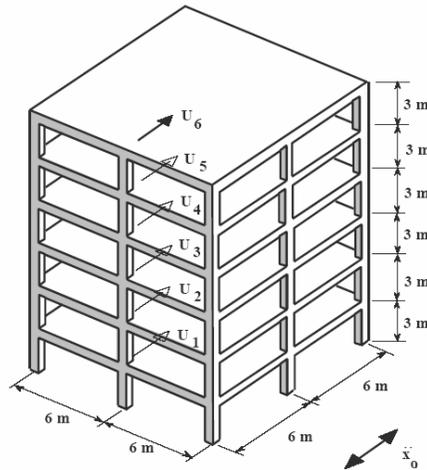
We want to study the response of the building to the N-S component of the recorded accelerations at El Centro, California, in May 18 of 1940.
